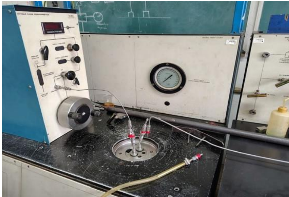
Fig. 3 - 11: Schematic photo of the arrangement used to measure V_p with gas.
