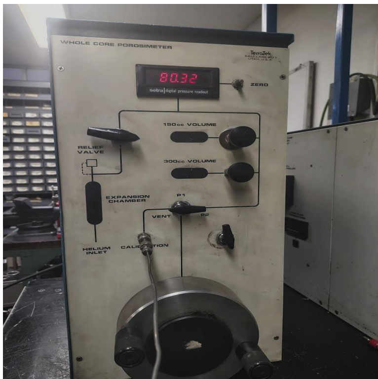
Fig. 3 - 10: Photograph of the porosimeter used at various experiment stages.
