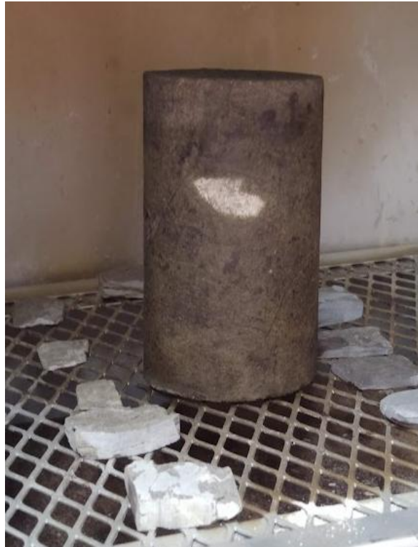
Fig. 3 - 5: Sample placed in a high-temperature oven to initiate the drying process.
