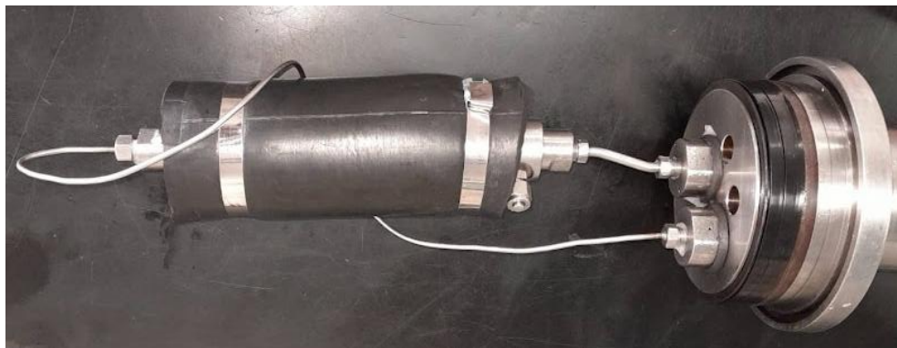
Fig. 3 - 6: The sleeved and assembled sample is ready for laboratory testing.
