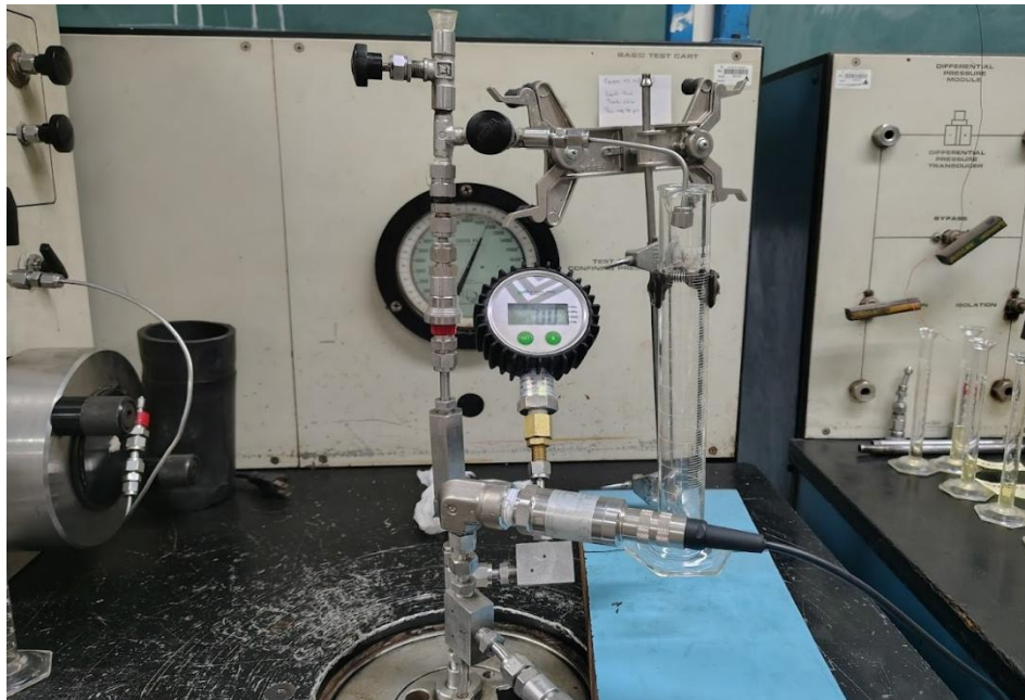
Fig. 3 - 22: Test tube added at the end of the setup to collect the volume expelled and/or recovered.
