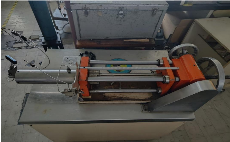
Fig. 3 - 8: Constant flow pump utilized for oil displacement and injection into the cores.
