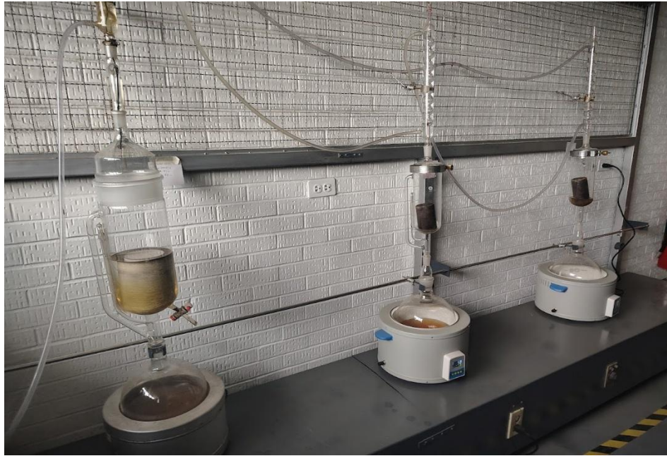
Fig. 3 - 4: The Dean-Stark apparatus is observed, where the sample washing process occurs.
