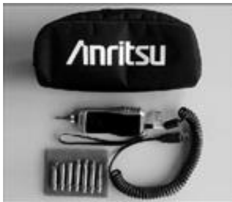
Figura 2.12. G0306A Video Inspection Probe (x400) [16].
