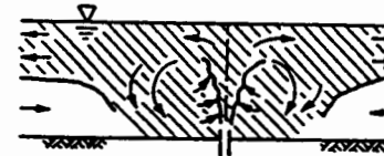
b) Shallow Water, Low Buoyancy, Vertical: Unstable Near-Field with Local Mixing and Restratification
