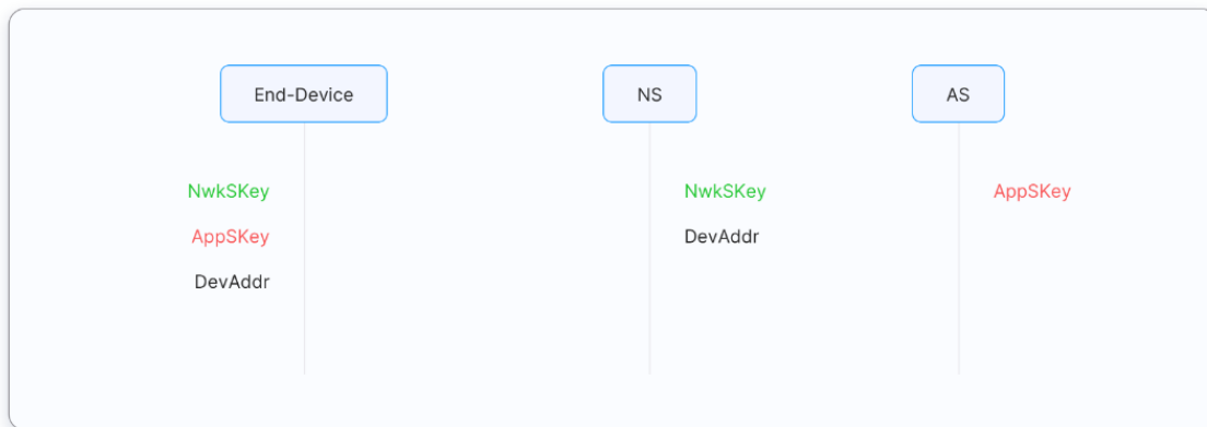
Figura 2.13: Mecanismo Activation by personalization [7].
