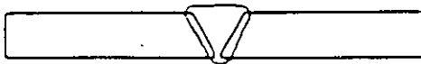
QW-463.1(b) PLATES — OVER \frac{3}{4} AND ALTERNATE \frac{3}{8} TO \frac{3}{4} IN. PROCEDURE QUALIFICATION
