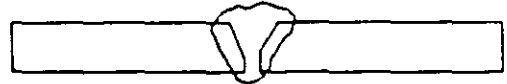
QW-463.2(b) PLATES — OVER \frac{3}{4} AND ALTERNATE \frac{3}{8} TO \frac{3}{4} IN. PERFORMANCE QUALIFICATION
