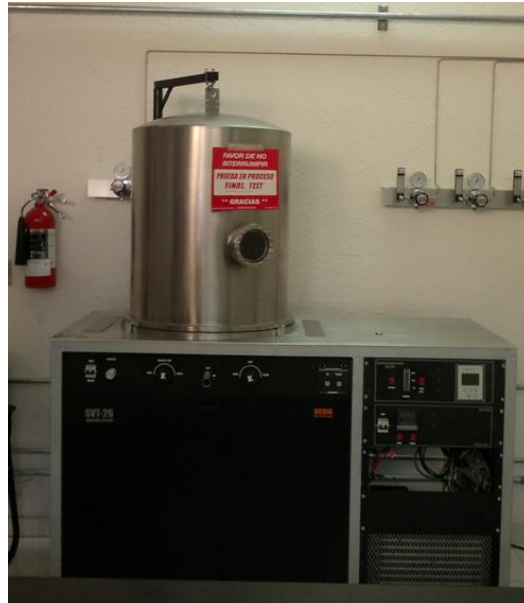
Figure81. Custom-made vacuum chamber.
