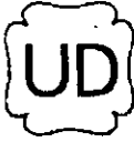
FIG. UG-129.2 OFFICIAL SYMBOL FOR STAMP TO DENOTE THE AMERICAN SOCIETY OF MECHANICAL ENGINEERS' STANDARD FOR RUPTURE DISK DEVICES
