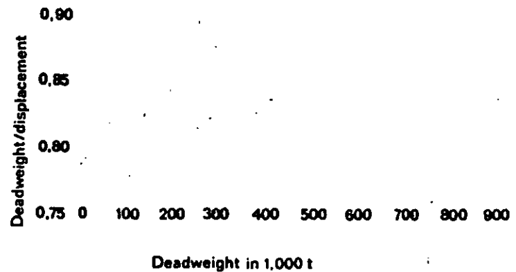
Fig. 158. Ratio of deadweight to displacement for tankers.
