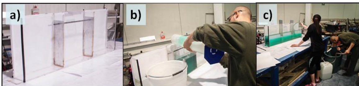
Figure 21. a) The gates were closed and sealed with wax; b) the center compartment was filled with dyed saltwater and the 2 remaining compartments with freshwater; and c) once the experiment was recorded, the water was taken out of the container.
