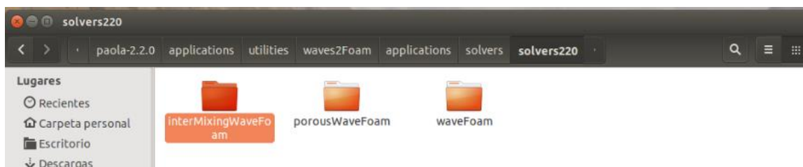
Figure 12. Location of the new solver named interMixingWaveFoam . The folder from the previous Figure was copied and pasted in this location on waves2Foam toolbox and its name was simply changed to interMixingWaveFoam .
