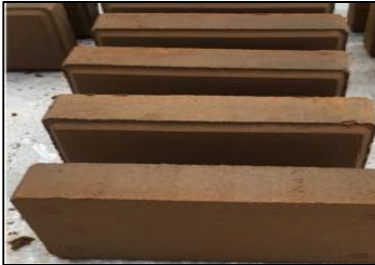
Figura 4. 16. Ladrillo conformado por cemento y jales IoT. Fuente: Technological properties of soil-cement bricks produced with iron ore mining waste (Pereira et al., 2019)
