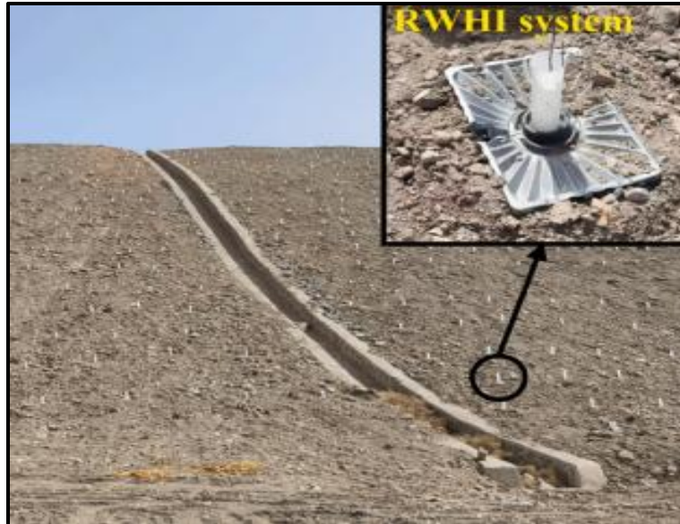
Figura 4. 32. Sistema RWHI en Wuda, China. Fuente: A new small-scale system of rainwater harvesting combined with irrigation for afforestation in mine area: Optimizing design and Application (Liu et al., 2022).
