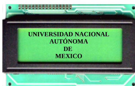
Figura 3.16 LCD 20 X 4 caracteres.
