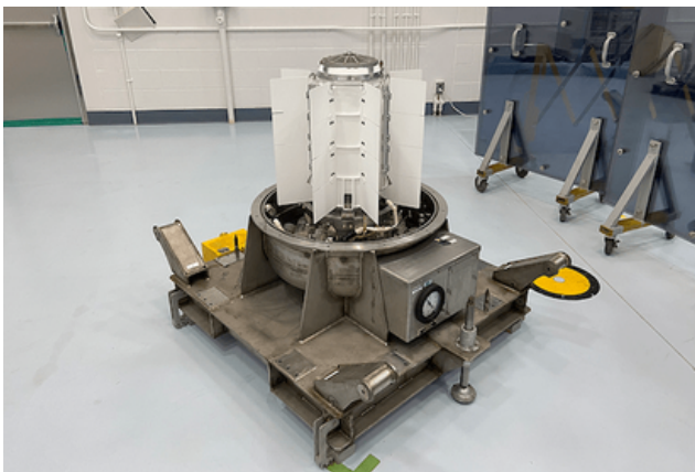
Figura 10.26 Reactor MMRTG del Perseverance
