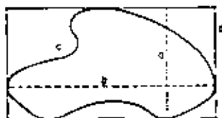
Fig. 2. Basic rectangle. (a) Minor axis of c . (b) Major axis of c . (c) Region. (d) Basic rectangle of c . The eccentricity e = b/a is always greater than or equal to 1. It is a shape descriptor, although not a good one.
