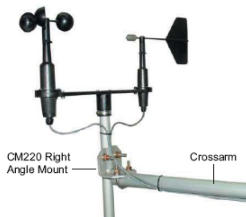
The 03001 is secured to one end of the CM206 Crossarm with the CM220 Right Angle Bracket.
