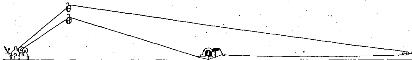
(c) THE DRAG SCRAPER CABLEWAY FOR DRAGGING AND STOCKPILING SOILS
