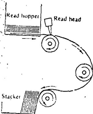
Fig. 10-3. Card-reading operation.
