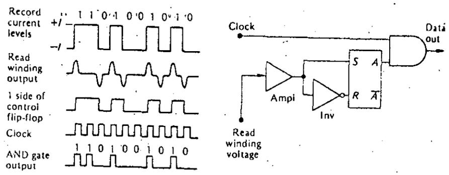
Fig. 10-12. NRZ recording and reading.
