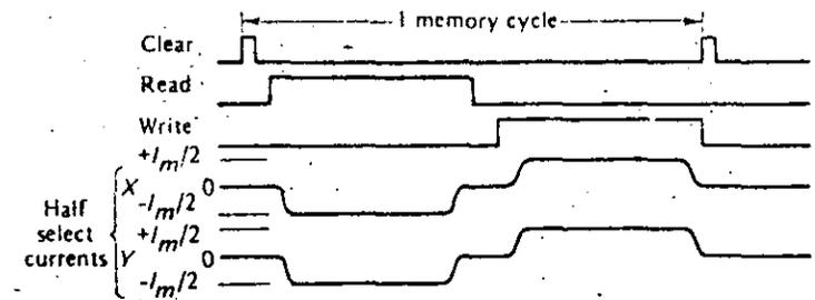
Fig. 12-17. NDRO waveforms for Fig. 12-16 (read from memory).
