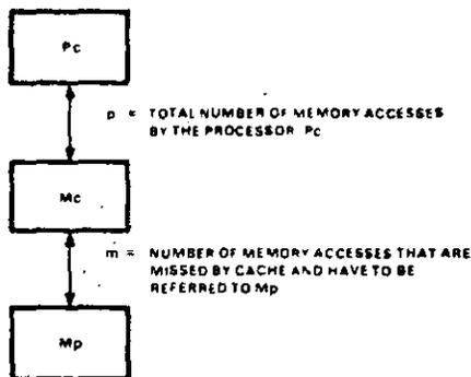
Figure 1. The structure of Pc, Mcache, and Mp of cached computer.
