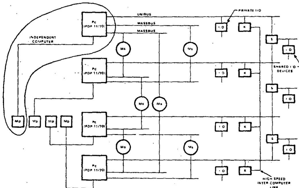
Figure 9. Four-processor multicomputer system based on PDP-11/70 processors.
