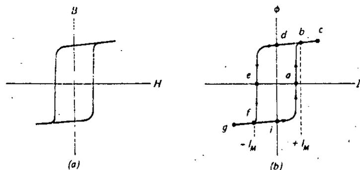
general shape. A plot of flux in the core  $\phi$  versus driving current  $I$  is shown in Fig. 12-2b. We shall base our discussion on this curve since it is generally easier to talk in terms of these quantities.
