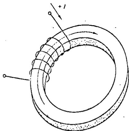
Fig. 12-1. Magnetic core.
