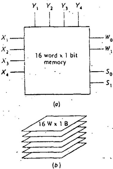
Fig. 12-24. (a) Logic diagram. (b) Six chips stacked to get a 16-word  $\times$  6-bit memory.
