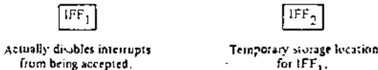
The state of IFF<sub>1</sub> is used to actually inhibit interrupts while IFF<sub>2</sub> is used as a temporary storage location for IFF<sub>1</sub>. The purpose of storing the IFF<sub>1</sub> will be subsequently explained.
