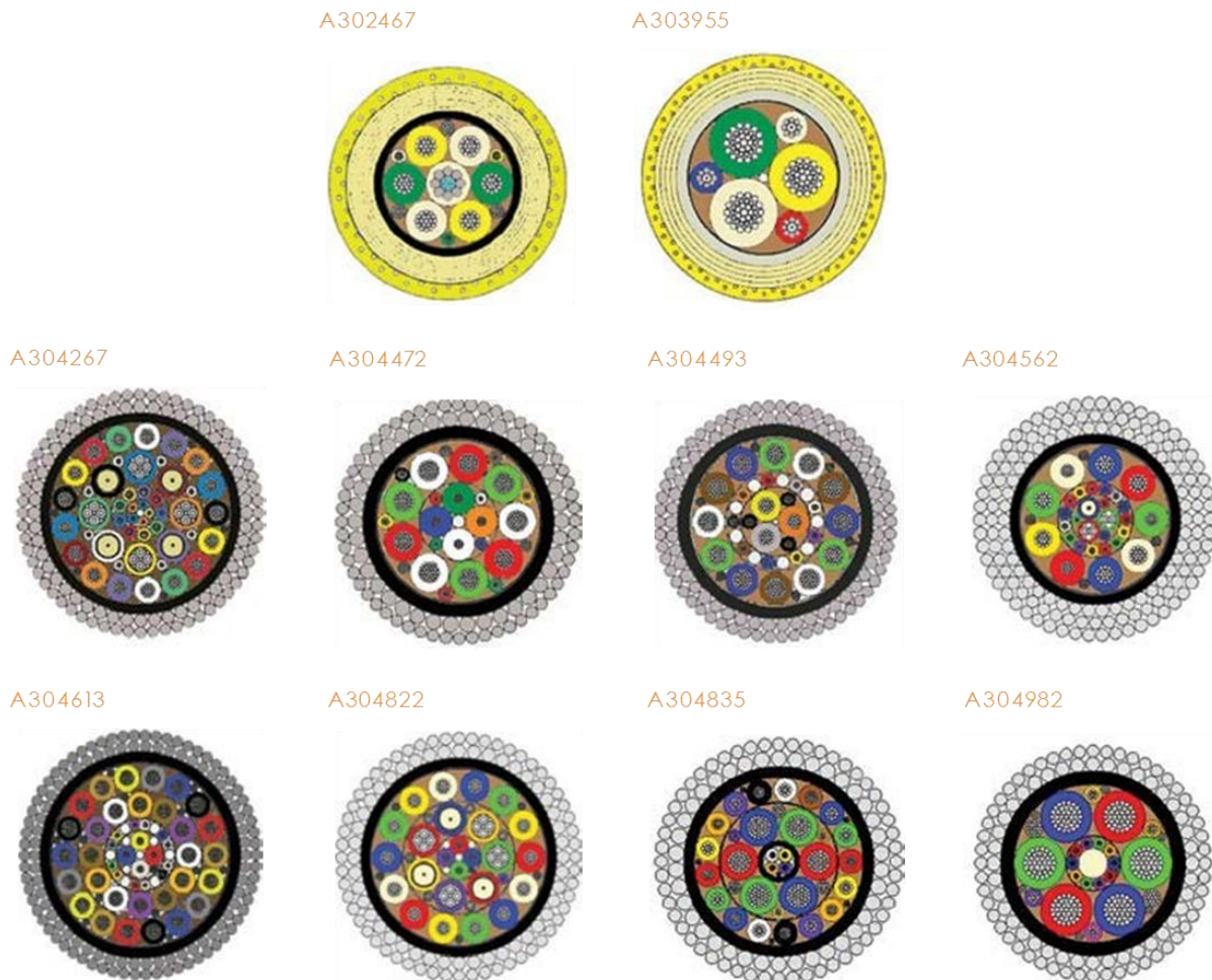
Figura 7 Secciones de cables umbilicales, cortesía de TEconnectivity Industries & Solutions Oil, Gas and Marine
