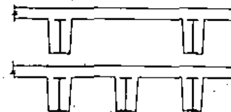
Fig. 1.15 Encased slab-and-beam system
