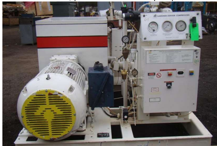
Figura II.75. Compresor Gardner Denver, [Cortesía ICA].
