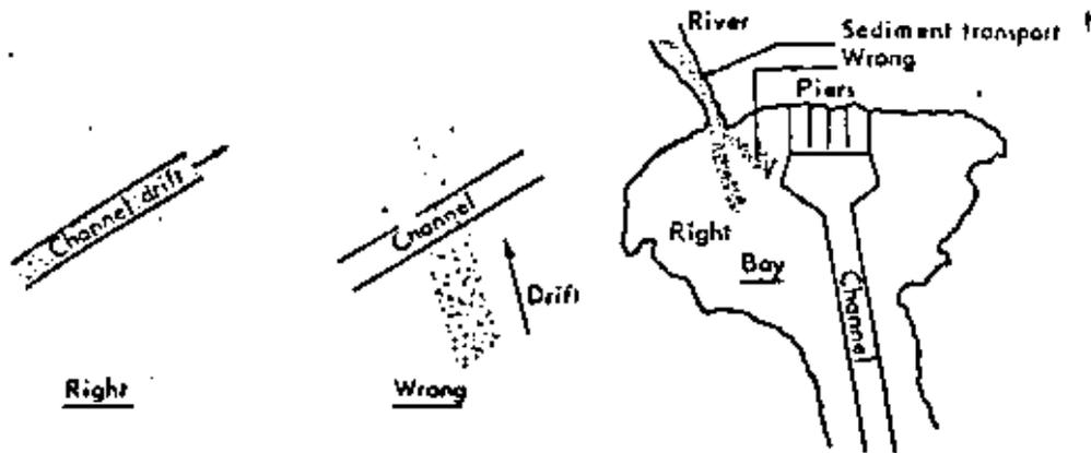
Figure E.1. Tracing pattern of drift at navigation channel; planning navigation channel; investigation of sedimentation at navigation channel.
