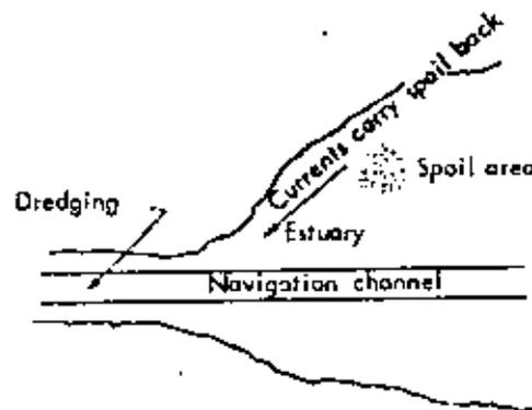
Figure E.11. Will spoil from dredging of navigation channel return to the channel?
