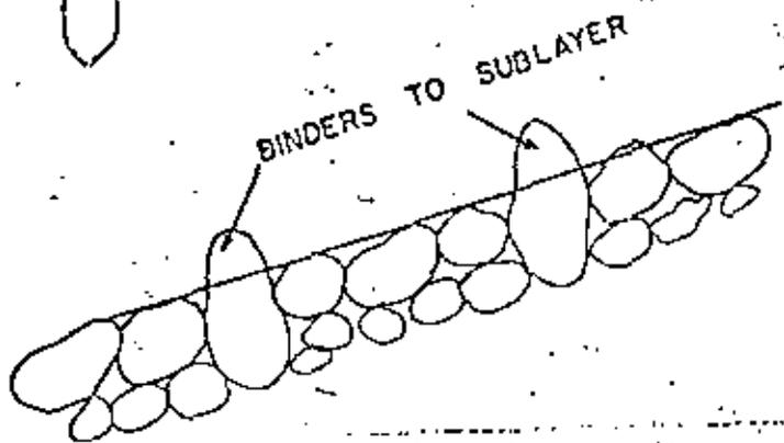
Fig. 6. How to roughen the first sublayer to provide better friction connection between armour and first sublayer (refs. 4 and 8). See also Appendix 7, Chapter 3.
