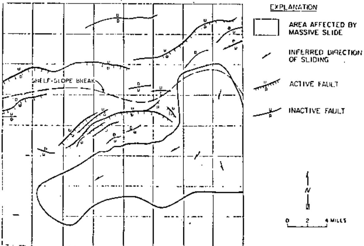
Figure 5: Generalised map of area south of Galveston, Texas, showing deep-seated growth faults and area affected by large, late Pleistocene slide. Group of curvilinear faults between shelf break and northern boundary of slide area is related to growth of a large salt ridge at depth. Each grid square covers an area equivalent to a USA standard lease block, about 5 square miles.
