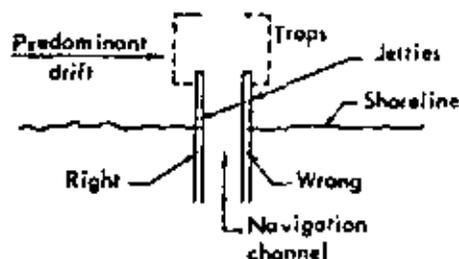
Figure E.7. Shall sand traps be placed symmetrically or asymmetrically at an entrance?
