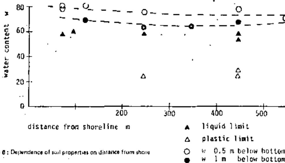
Figure 6: Dependence of soil properties on distance from shore
