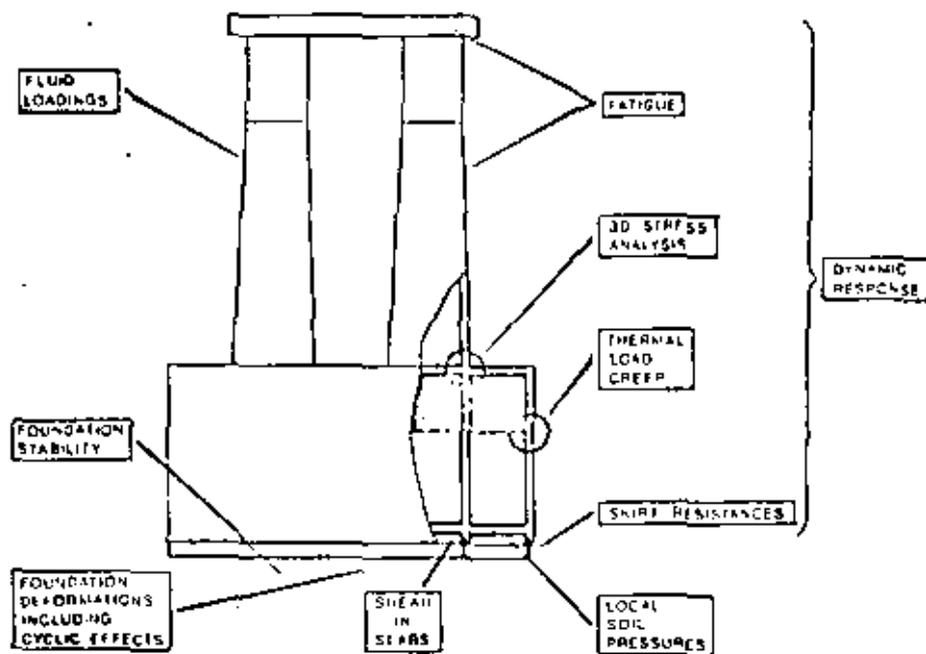
Figure 1.13 Current analytical problem areas for gravity platforms
