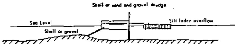
Figure E.18. Overflow of silt-laden water from sand and gravel dredge or shell dredge.
