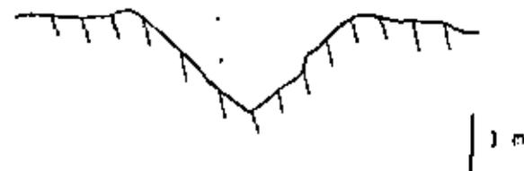
Figure 3: Trench section obtained by high frequency profiler
