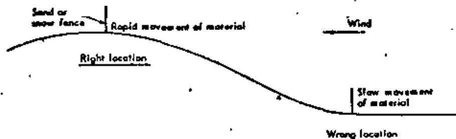
Figure E.19. Where should a sand fence be located to assure highest efficiency? Where does the material come from?
