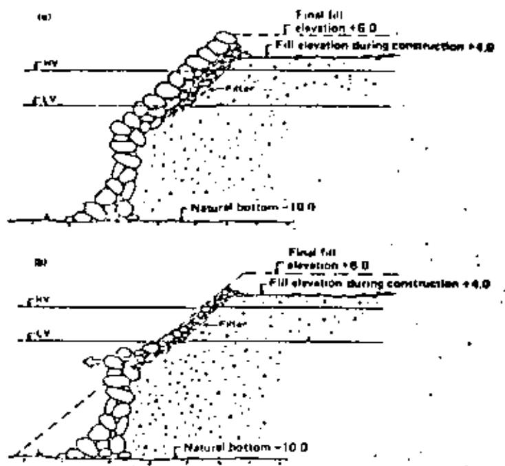
Fig. 12. A. An unstable break water head, built up on a steep slope below water.
