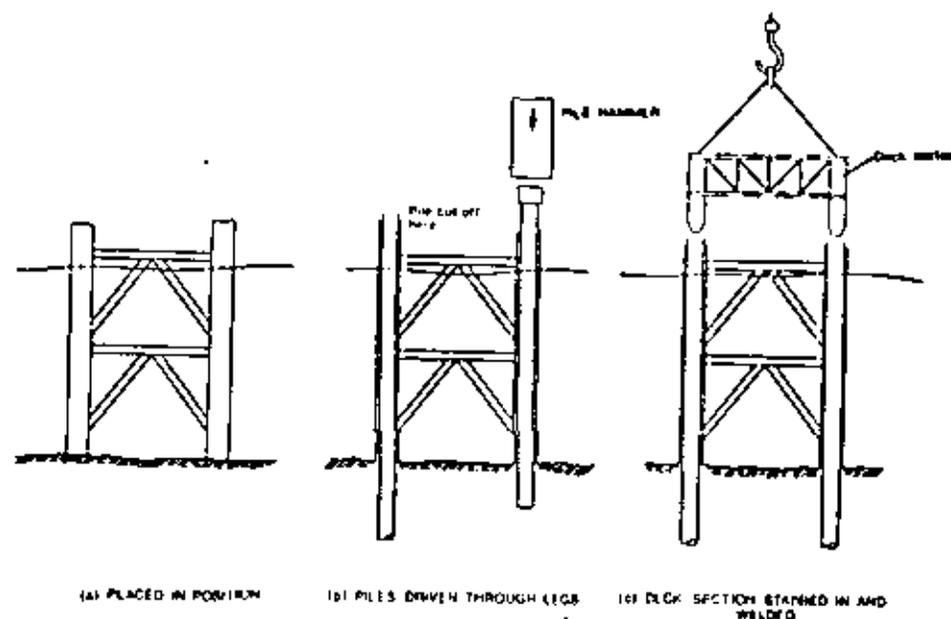
Figure 1.2 Principle of jacket or template
