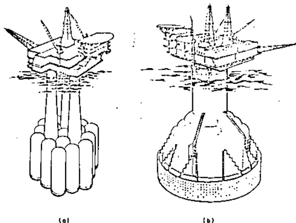
Figure 1.5 Concrete gravity platforms. (Reproduced by permission of Inst. Civil Eng.)
