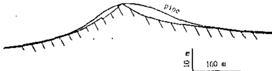
Figure 2: Section through sand wave (vertical exaggeration 5 : 1)
