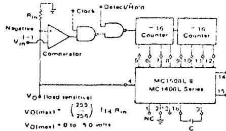
FIGURE 31 - PROGRAMMABLE PULSE GENERATION
