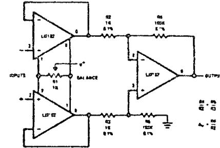
Differential Input Instrumentation Amplifier
