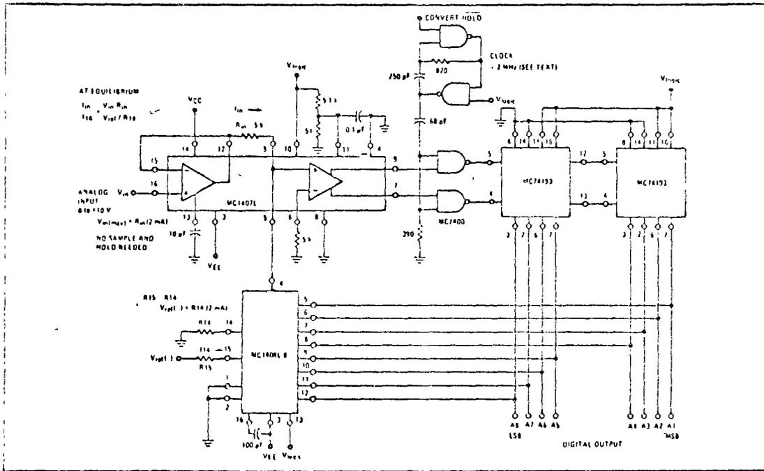
FIGURE 35 - 8 BIT TRACKING A TO D CONVERTER
