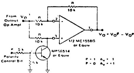
Programmable Gain Amplifier or Digital Attenuator
