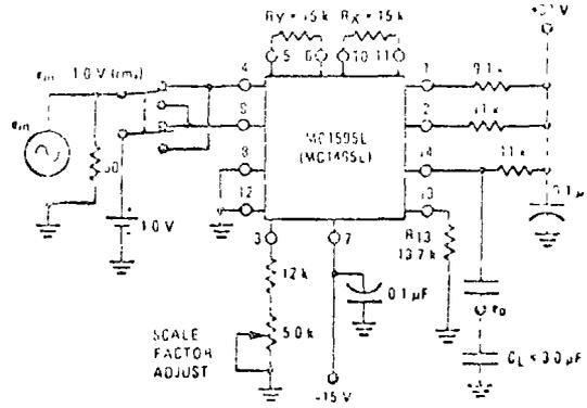
FIGURE 10 - BANDWIDTH ( $R_L = 50 \text{ }\Omega$ )
