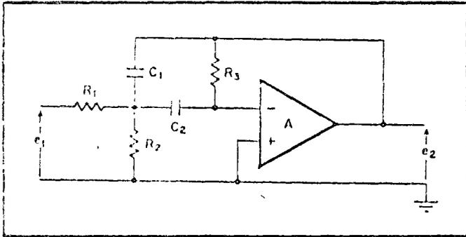
1. Basic network. This active bandpass RC filter provides two feedback paths via  $R_3$  and  $C_1$  for precise trade-off control between gain response and phase shift. The circuit also keeps component count low. When  $R_2$  is very large compared to  $R_1$ , it can be omitted altogether.
