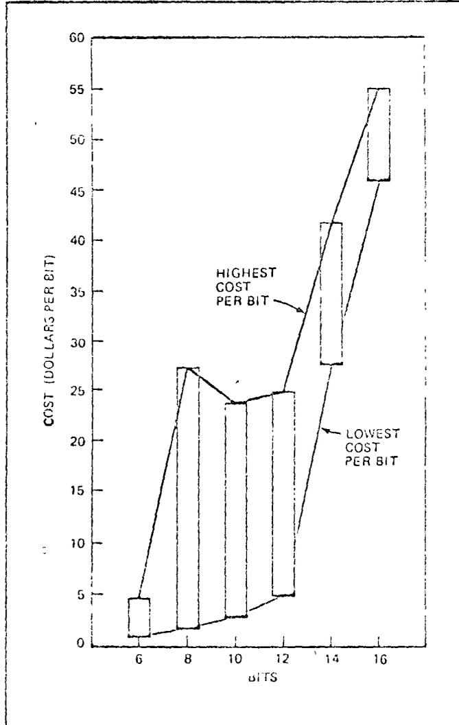
**2. Premium.** Cost-per-bit data, based on Fig. 1, emphasizes the cost increment for attaining and maintaining DAC precision. The gradual price increase for lesser-bit DACs results from volume production and less stringent demand on component tolerances.
