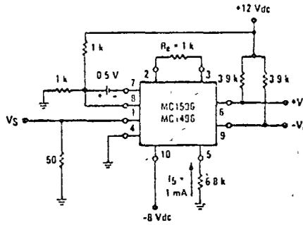
Pin number references pertain to this device when packaged in a metal can. To ascertain the corresponding pin numbers for a ceramic packaged device refer to the PIN CONNECTION CHART on the first page of this specification.
