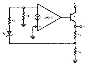
d) Regulating  $V_0$  by Adding Temperature Compensation
