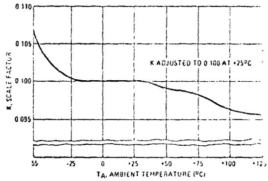
FIGURE 17 - ERROR CONTRIBUTED BY INPUT DIFFERENTIAL AMPLIFIER
