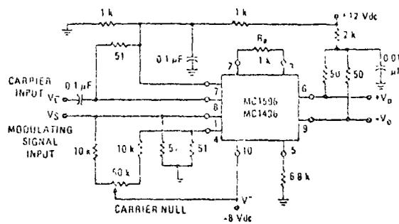
Pin number references pertain to this device when packaged in a metal can. To ascertain the corresponding pin numbers for a ceramic packaged device, refer to the PIN CONNECTION CHART on the first page of this specification.
