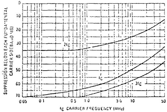
FIGURE 21 - CARRIER FEEDTHROUGH versus FREQUENCY
