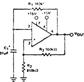
\*Chosen for oscillation at 100Hz
