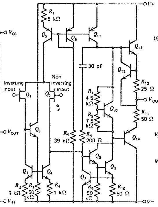
$\mu$ A740A Schematic Diagram
