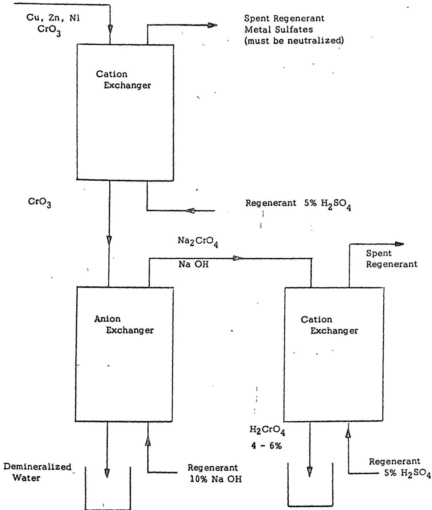
Figure 3 Schematic of ion exchange for chromate and water recovery.
