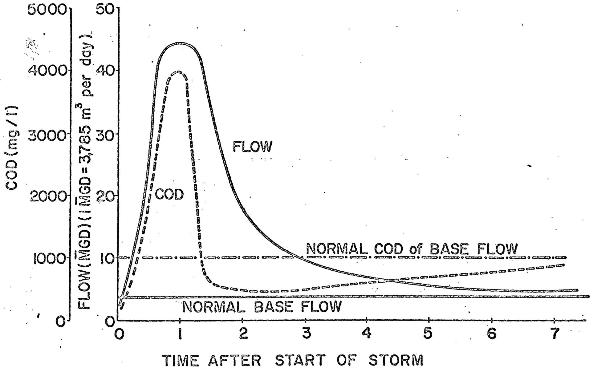
FIG. 4. STORM RUNOFF FLOW AND QUALITY CHARACTERISTICS FOR TYPICAL REFINERY / PETROCHEMICAL INSTALLATIONS.
