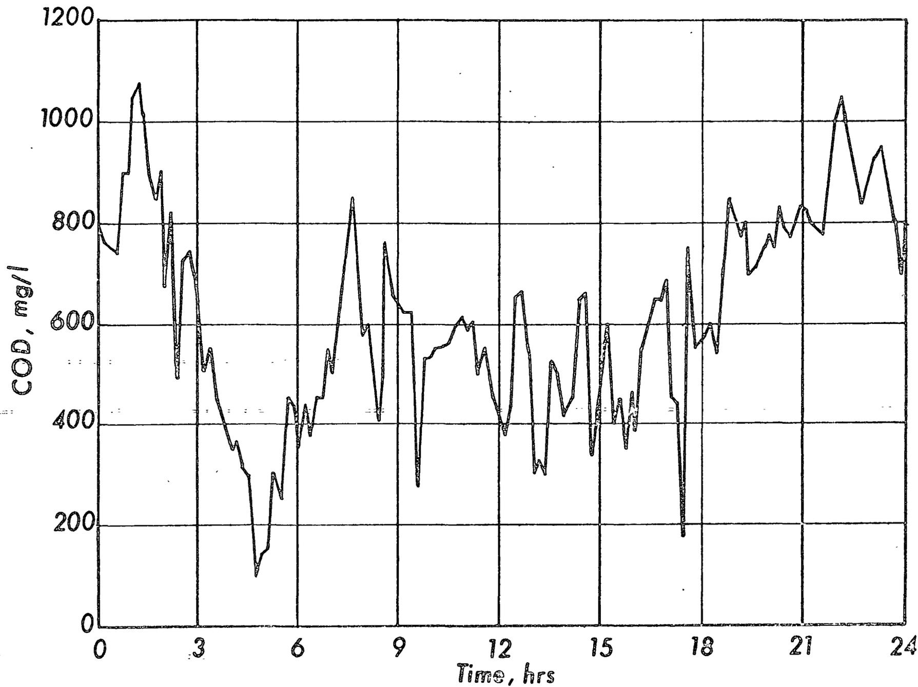
Figure 2 - Typical  $\text{COD}$ -Concentration Curve
