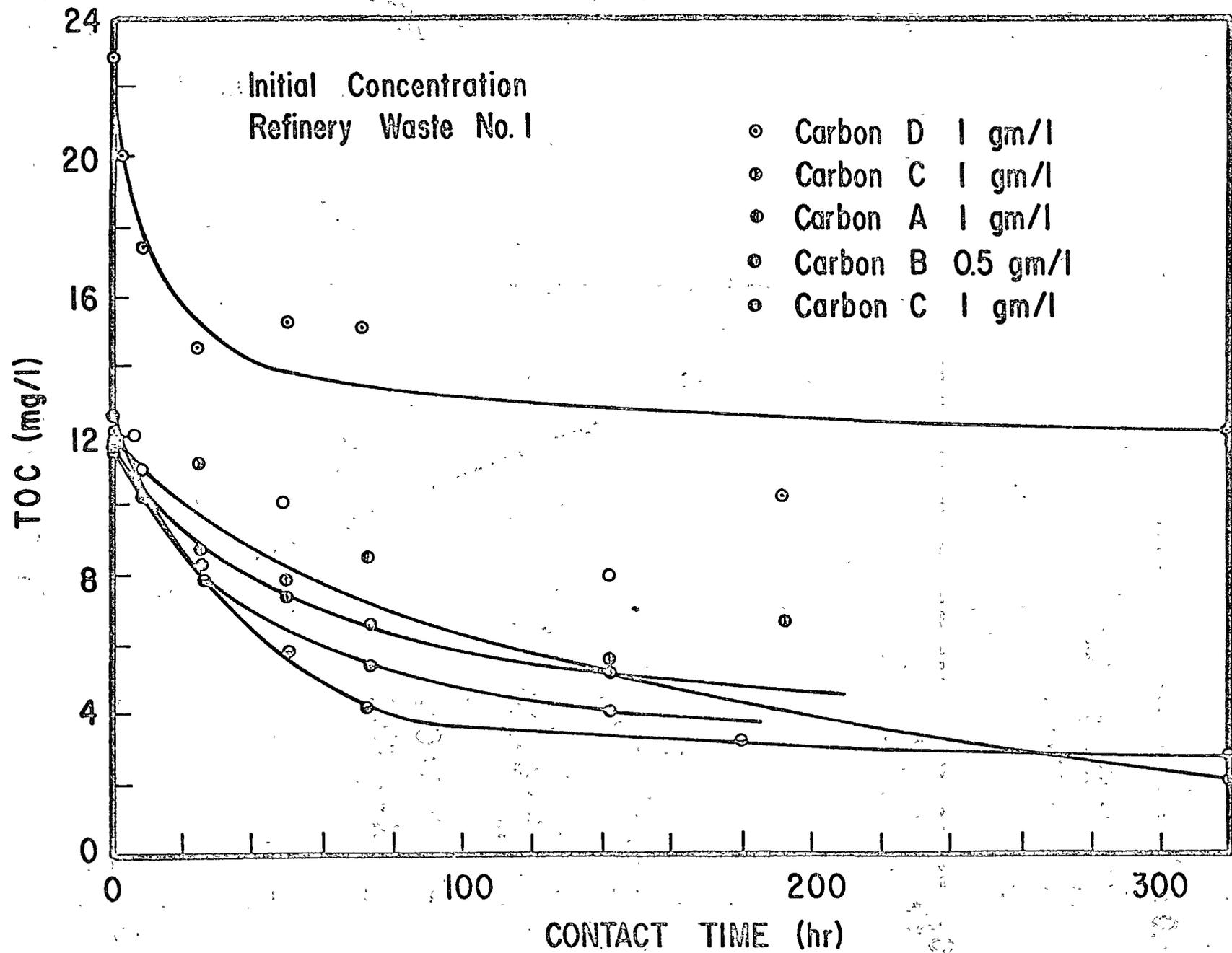
FIG. 4 - REDUCTION OF ORGANIC CARBON IN REFINERY WASTEWATER
