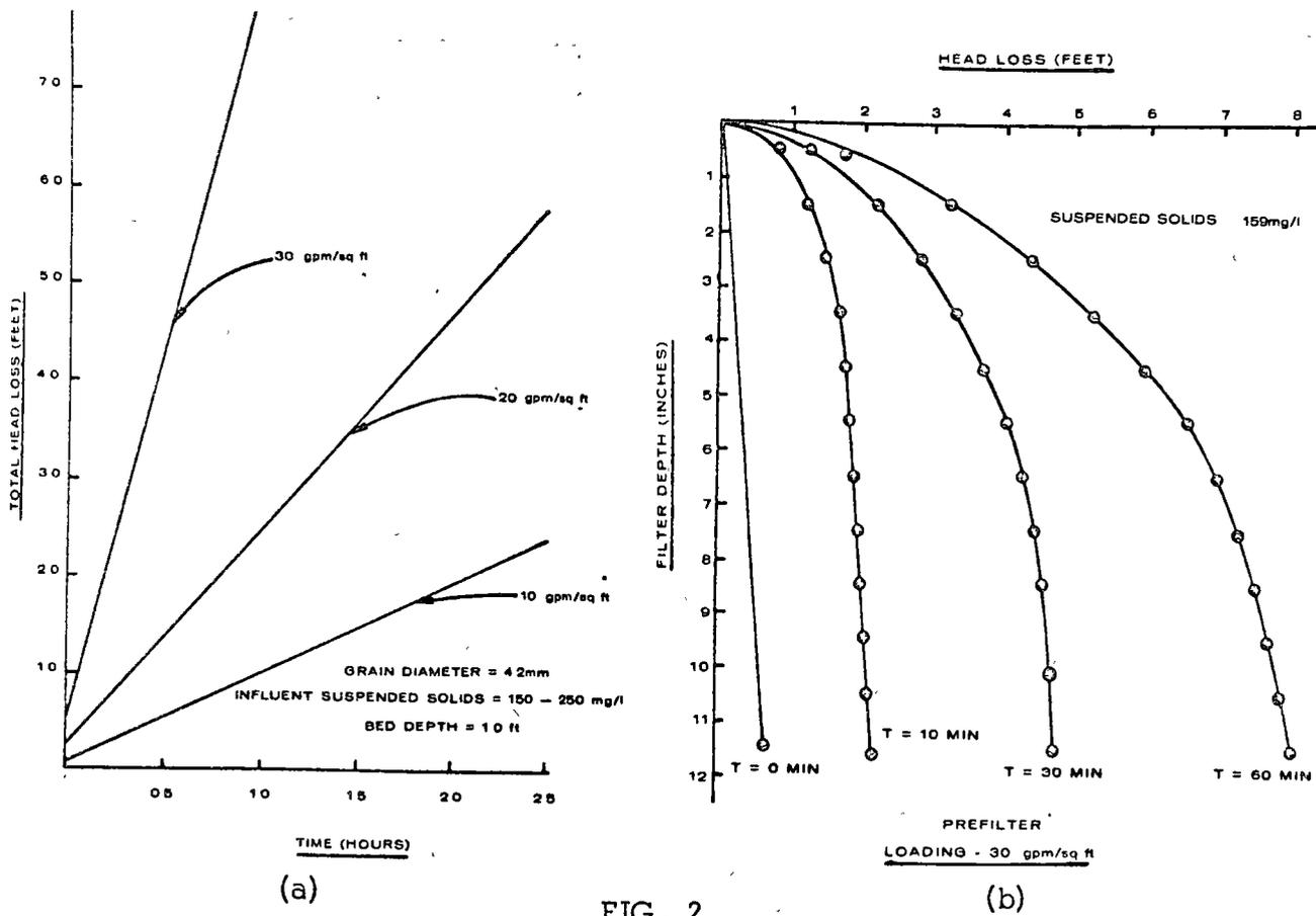
FIG. 2 Headloss-Depth-Time Relationship for PVC Pellets
