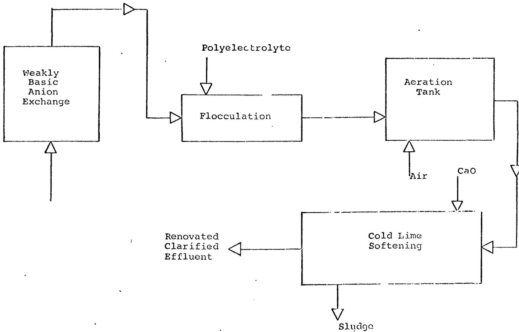
... - Modified DESAL Process for Treatment of Secondary Municipal Effluent
