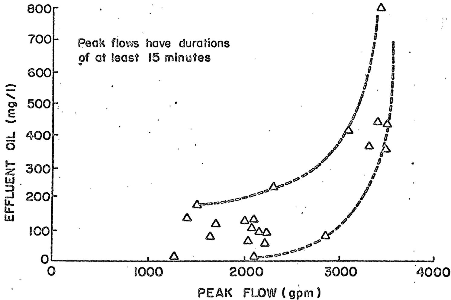
FIG. 6. INFLUENCE OF PEAK FLOWS ON EFFLUENT OIL CONCENTRATION.
