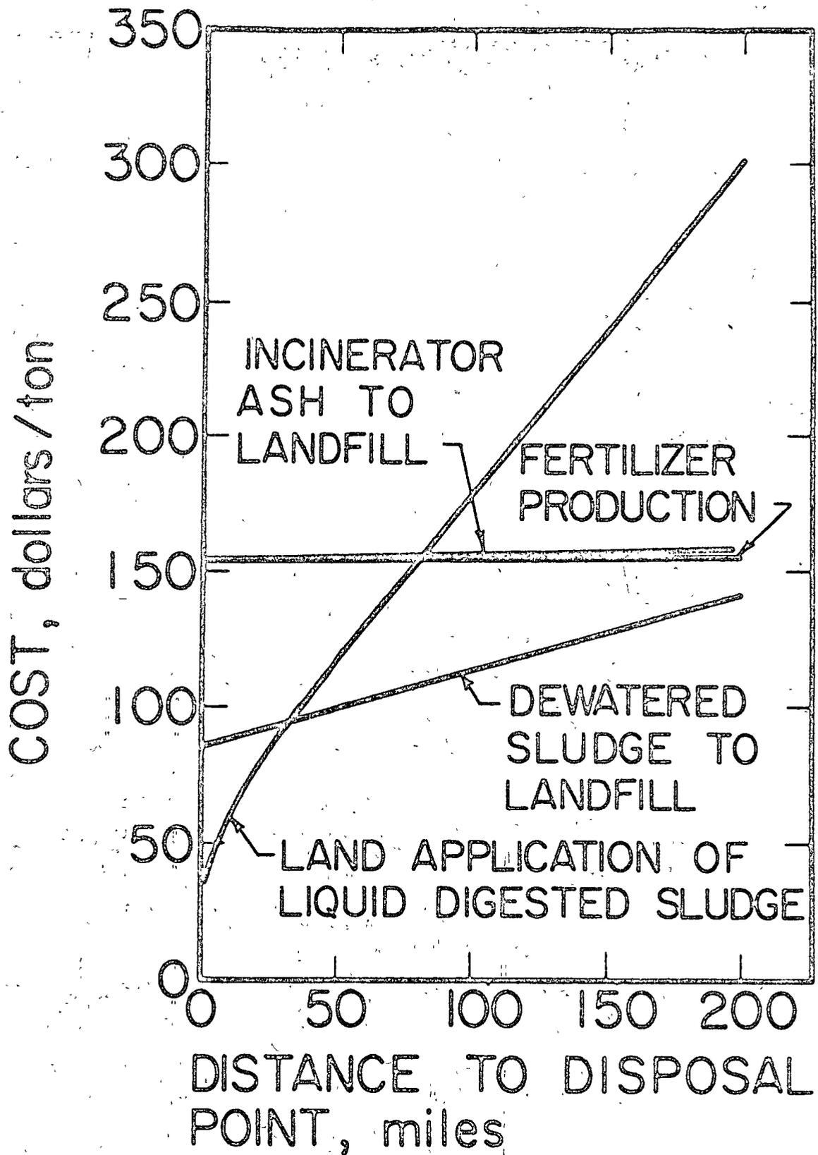
FIGURE 1. COST OF DISPOSAL OF APPROXIMATELY 5000 gpd OF SLUDGE BY VARIOUS METHODS. (CITY OF 10,000 PEOPLE - AFTER RIDDELL AND CORMACK, 1966).
