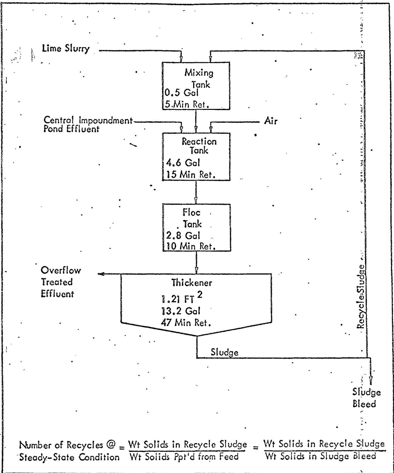
FIGURE 3 LAB SCALE SIMULATION OF CIP EFFLUENT TREATMENT FLOW DIAGRAM
