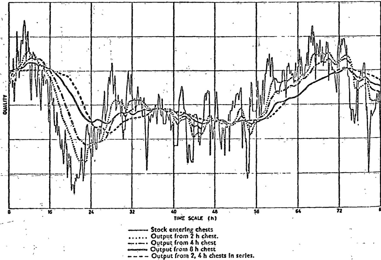
Fig. 2.—Results of computations of two, four, and eight-hour chests
