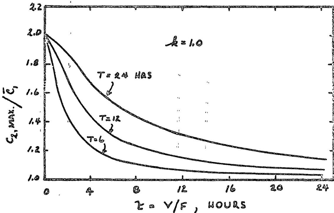
EQUALIZATION BASIN RESPONSE TO SINUSOIDAL INPUTS -
