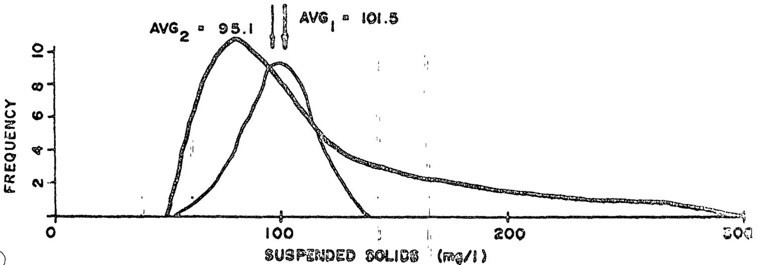
FIGURE 6 - EFFECT OF EQUALIZATION ON PRIMARY EFFLUENT
