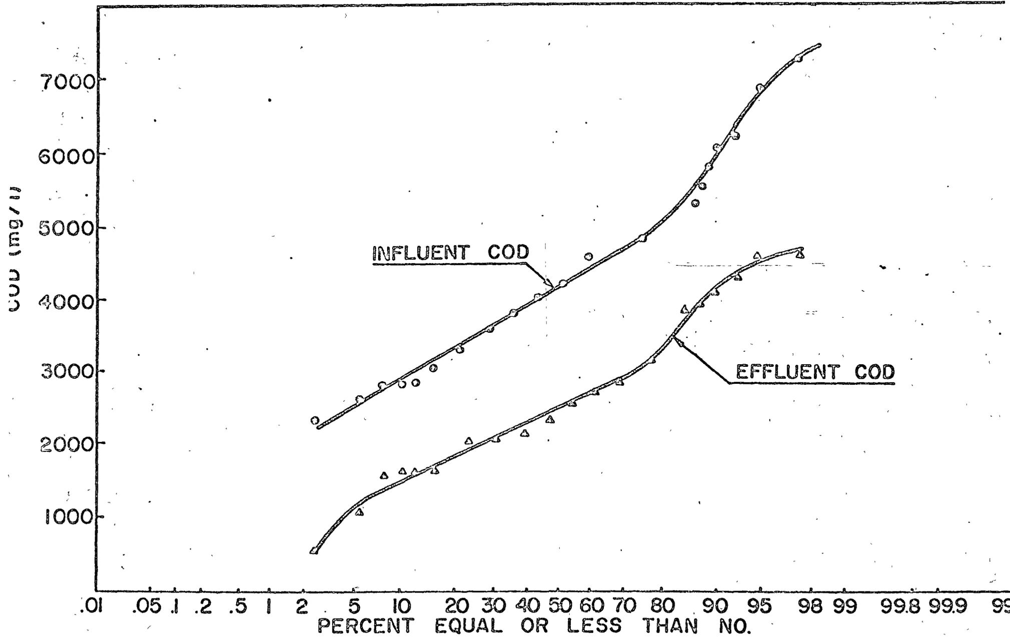
FIG. 9. EFFECTIVENESS OF PRIMARY TREATMENT FOR INTEGRATED REFINERY / PETROCHEMICAL FACILITY.
