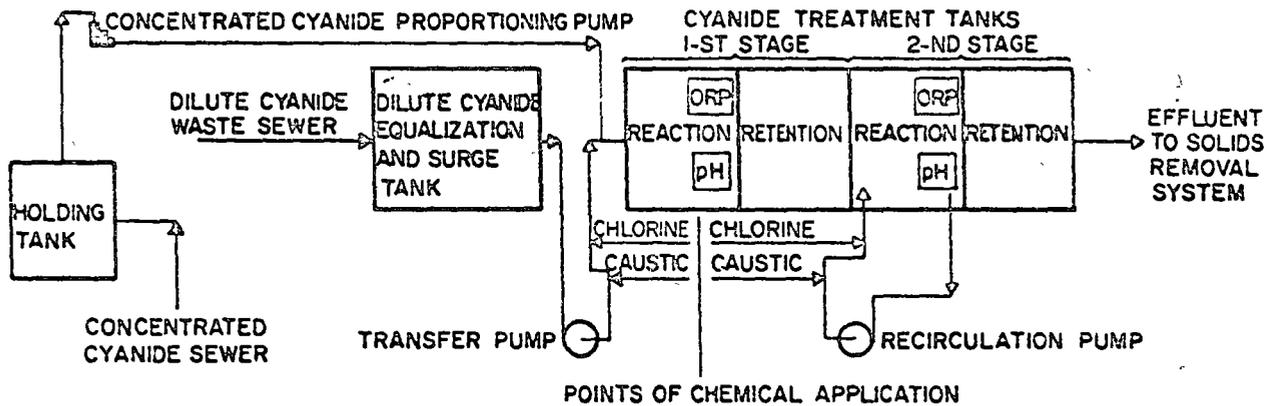
FIG. 2. CYANIDE WASTES CAN ALSO BE TREATED BY THE FLOW THRU TYPE PROCESS AS SHOWN IN THE SCHEMATIC DIAGRAM.
