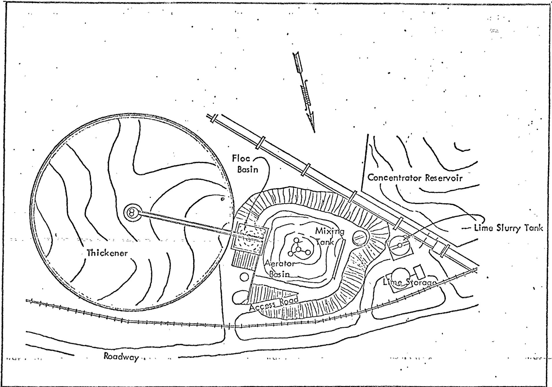
FIGURE 5 SKETCH OF CENTRAL TREATMENT PLANT
