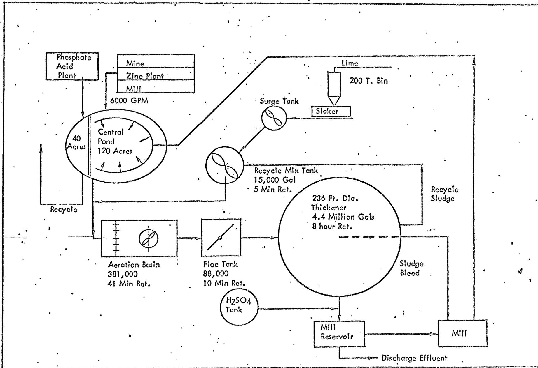
FIGURE 4 CENTRAL TREATMENT PLANT - FLOW SHEET
