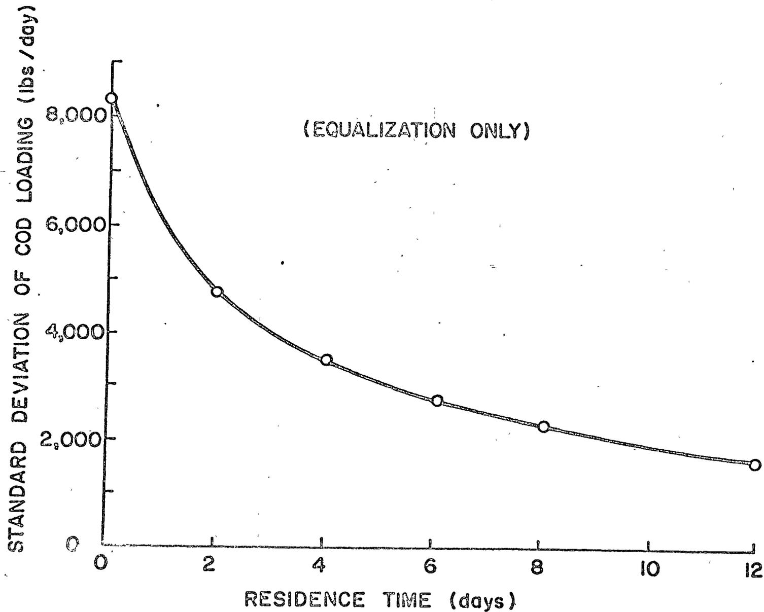
FIG. 5. STATISTICAL EVALUATION OF EQUALIZATION EFFICIENCY.
