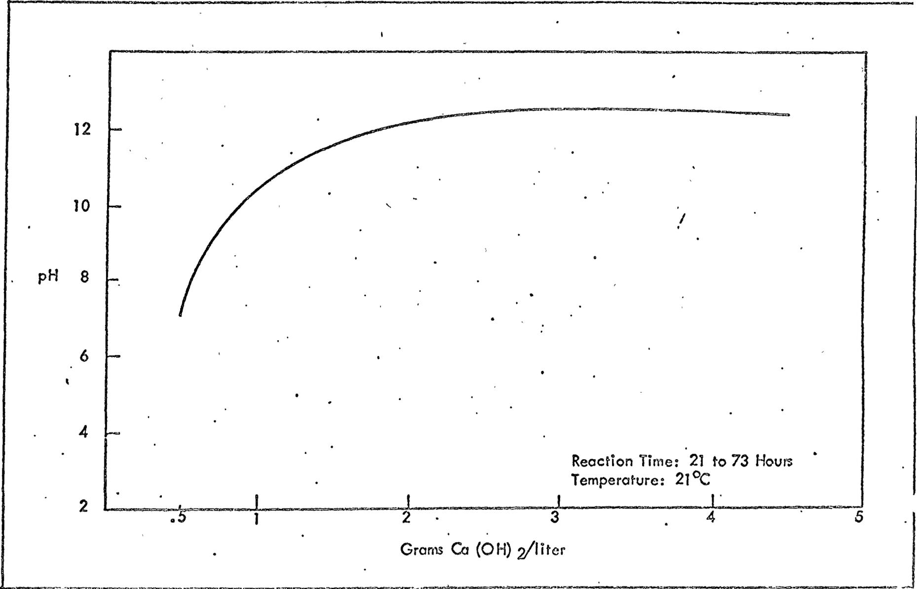
FIGURE 2. LIME CONSUMPTION vs pH for CENTRAL IMPOUNDMENT POND EFFLUENT
