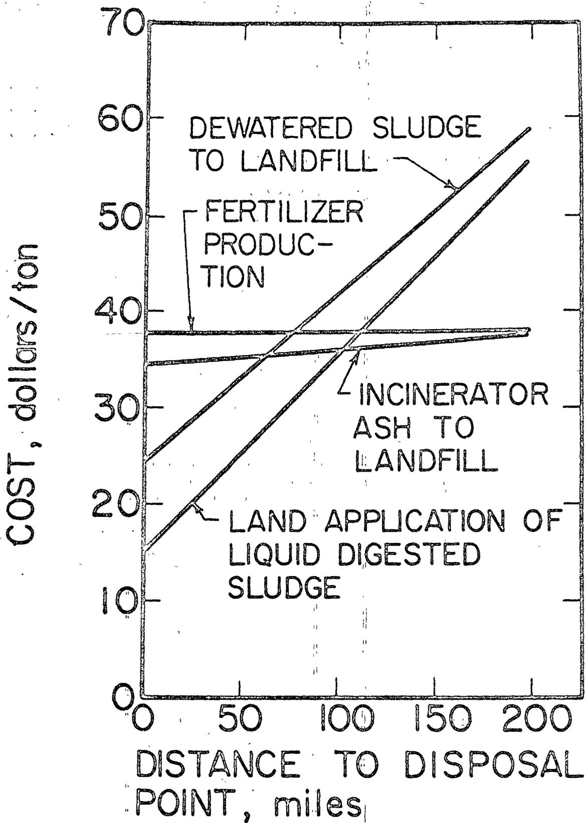
FIGURE 3. COST OF DISPOSAL OF APPROXIMATELY 500,000 gpd OF SLUDGE BY VARIOUS METHODS (CITY OF 1,000,000 PEOPLE - AFTER RIDDELL AND CORMACK, 1966).
