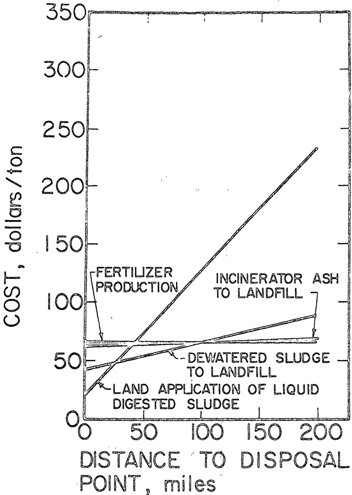
FIGURE 2. COST OF DISPOSAL OF APPROXIMATELY 50,000 gpd OF SLUDGE BY VARIOUS METHODS (CITY OF 100,000 PEOPLE - AFTER RIDDELL AND CORMACK, 1966).
