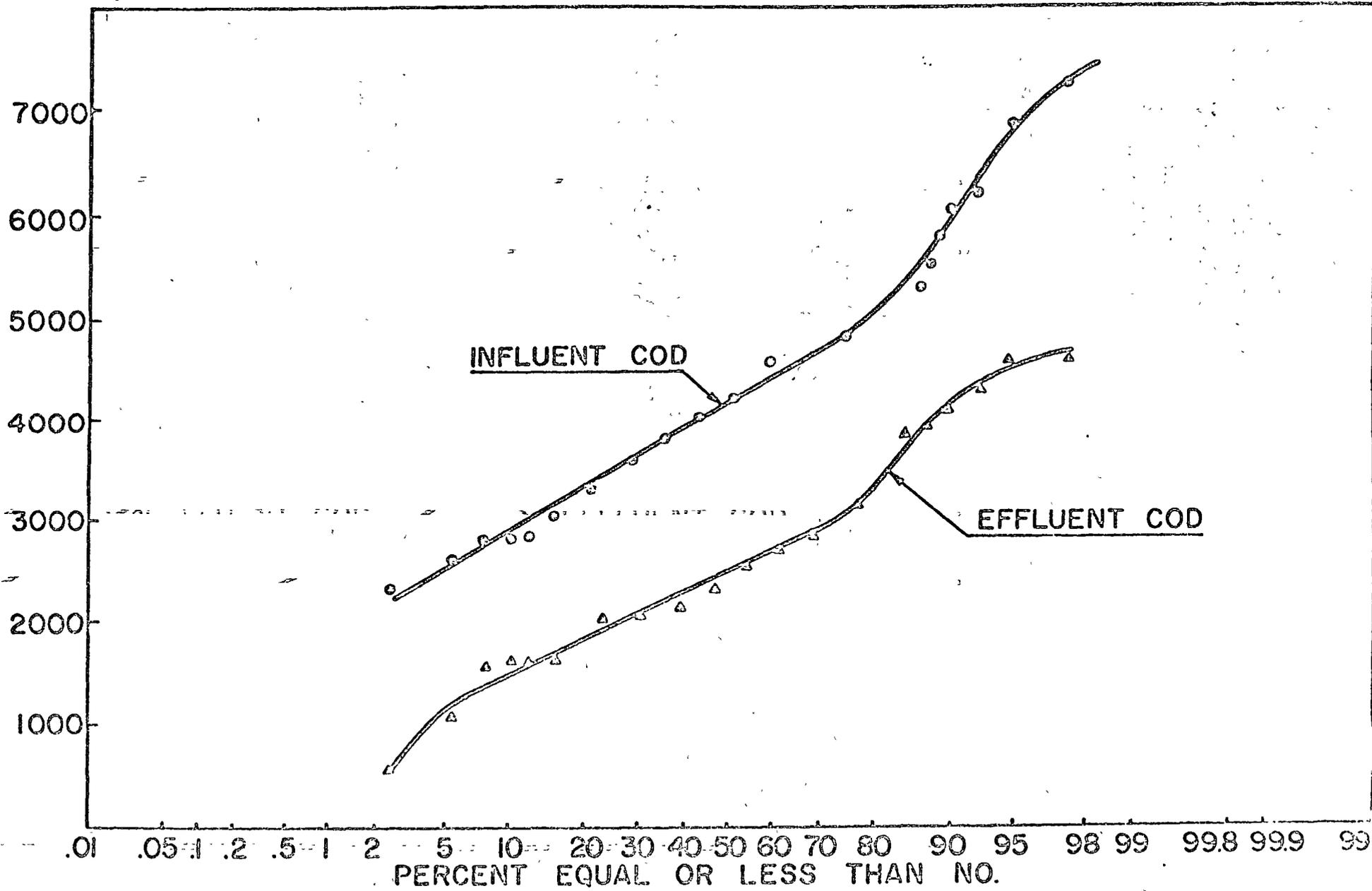
FIG.5. EFFECTIVENESS OF PRIMARY TREATMENT FOR INTEGRATED REFINERY / PETROCHEMICAL FACILITY.
