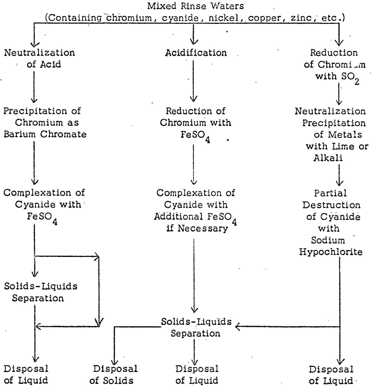
FIG. 4. PROCESSES APPLICABLE TO MIXED CHROMIUM AND CYANIDE RINSE WATERS
