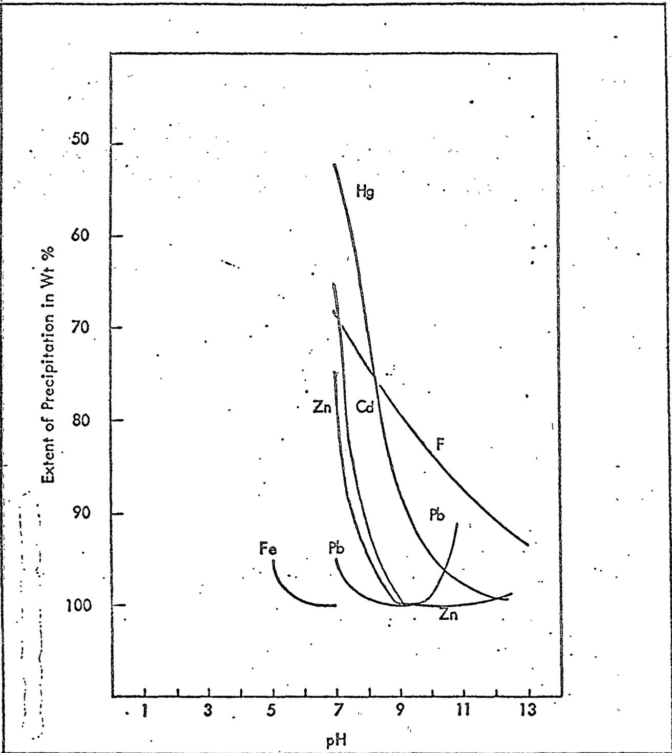
FIGURE 1 HEAVY METAL PRECIPITATION vs pH for CENTRAL IMPOUNDMENT POND EFFLUENT - pH ADJUSTMENTS BY LIME ADDITIONS
