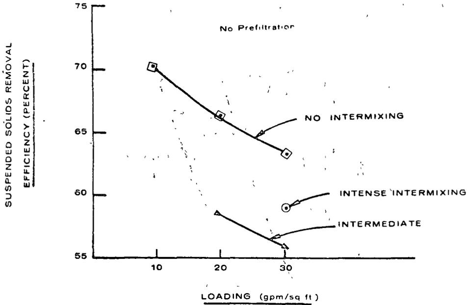
FIG. 5 Efficiency of Multilayered Filtration of Raw Sewage
