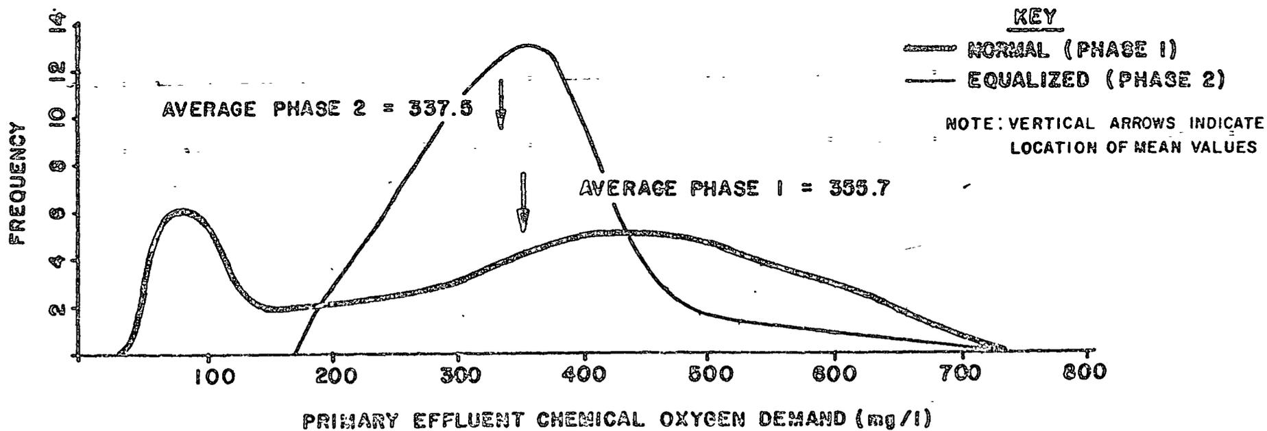
**FIGURE 5 EFFECT OF EQUALIZATION ON PRIMARY EFFLUENT DATA FROM DIURNAL SAMPLING SERIES**
