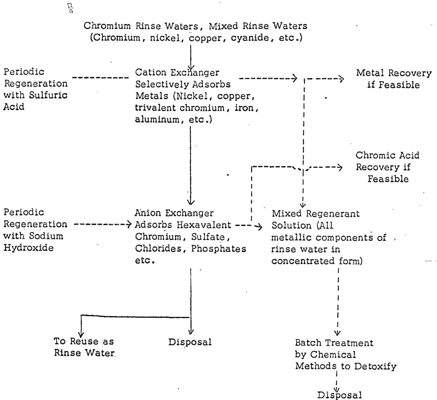
FIG. 5. ION EXCHANGE METHOD OF TREATING CHROMIUM RINSE WATERS OR MIXED RINSE WATERS
