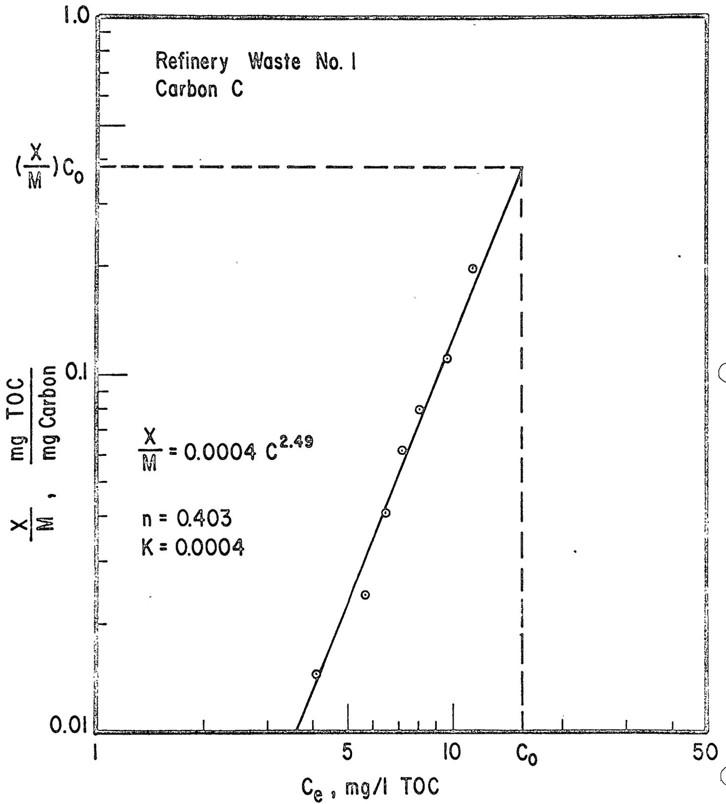
FIG. 5 - ADSORPTION ISOTHERM
