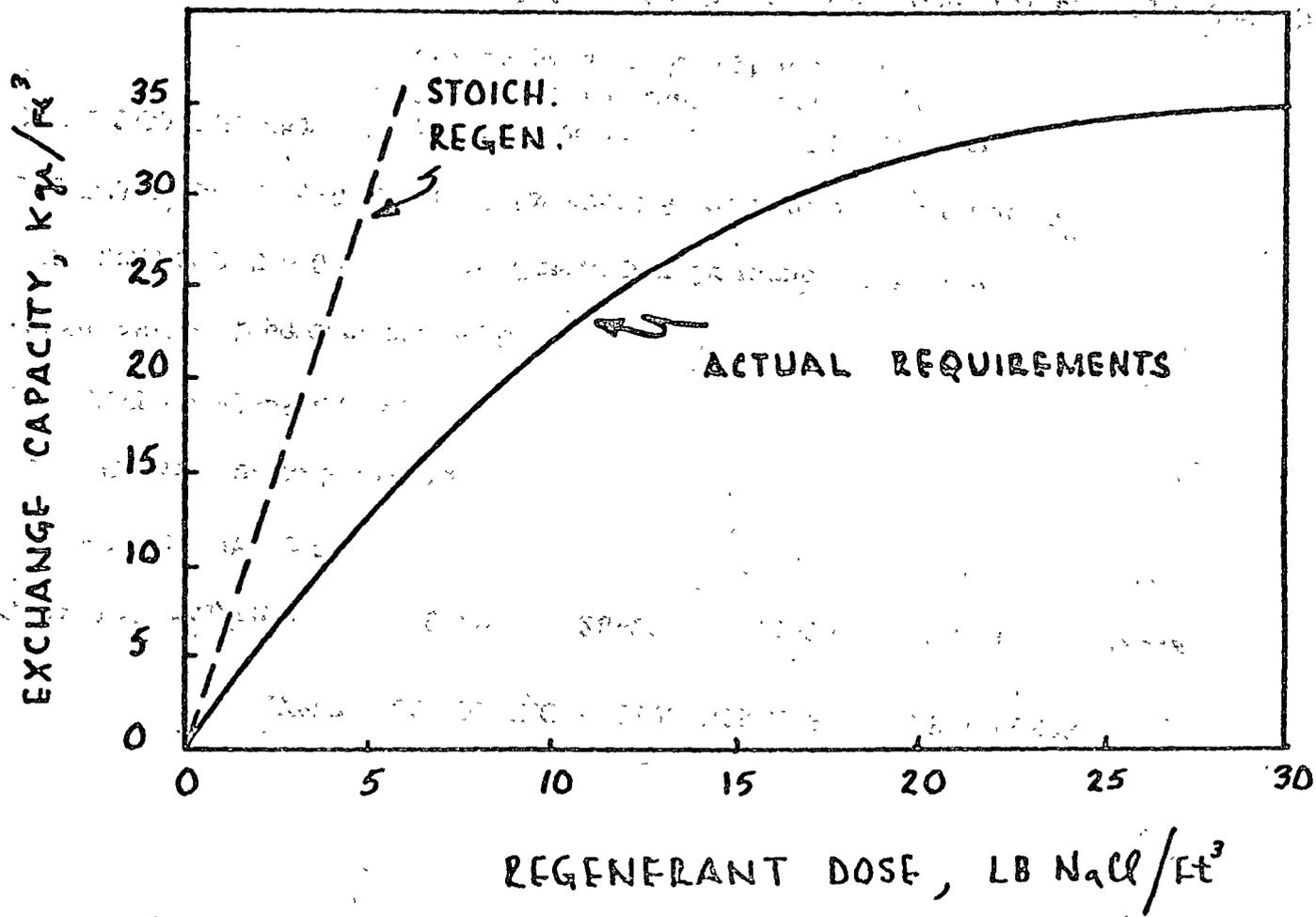
TYPICAL SOFTENING EXCHANGER DESIGN PARAMETERS
