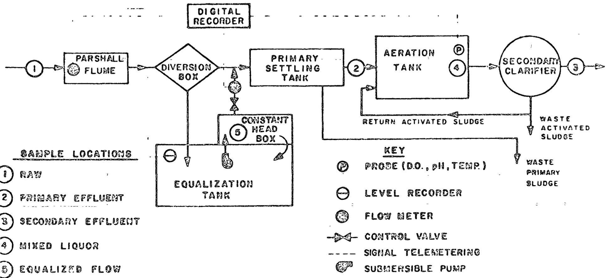
FIGURE 1 SCHEMATIC DIAGRAM OF FACILITIES
