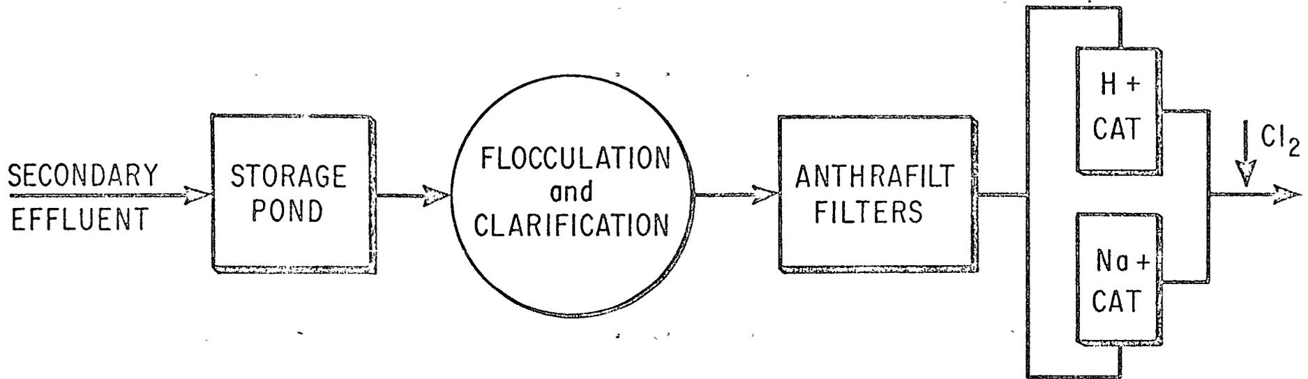
FIG. 3. WATER RENOVATION PROCESS – EL PASO PRODUCTS, TEXAS
