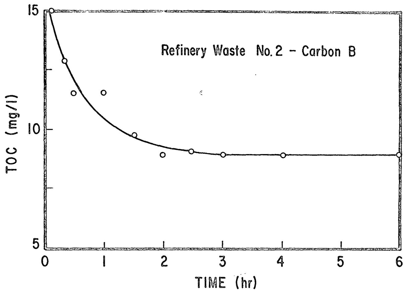
FIG. 1 - ADSORPTION RATE - PULVERIZED ACTIVATED CARBON
