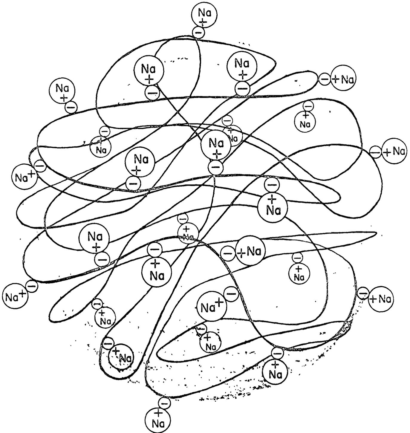
Model of a cation exchanger, showing negatively charged exchange sites on the skeleton holding sodium ions like grapes on a vine.
