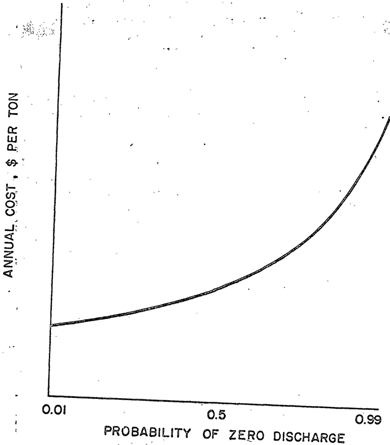
FIG. 2. RELATIONSHIP BETWEEN COST AND PROBABILITY OF ZERO DISCHARGE
