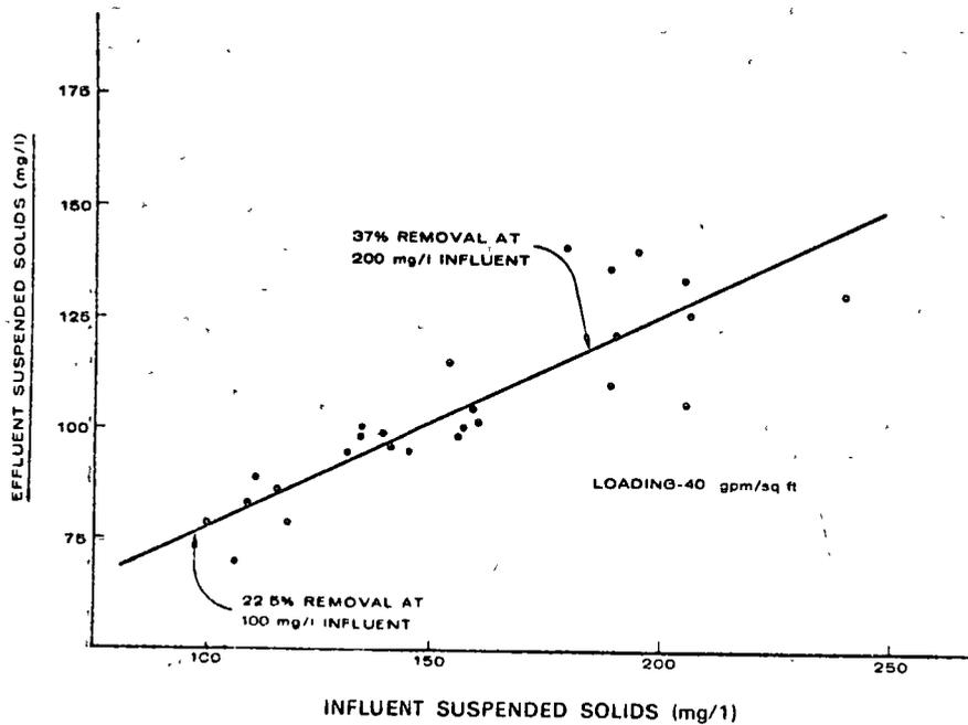
FIG. 3 Suspended Solids Removal by PVC Pellets
