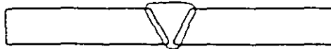
QW-463.1(b) PLATES — OVER \frac{1}{4} IN. AND ALTERNATE \frac{3}{8} TO \frac{1}{4} IN. PROCEDURE QUALIFICATION
