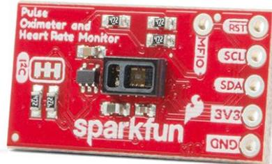
Fig. 26. Sensor de PPG. Recuperada de: [https://cdn.sparkfun.com/assets/parts/1/3/6/6/4/15219-SparkFun\\_Pulse\\_Oximeter\\_and\\_Heart\\_Rate\\_Sensor\\_-\\_MAX30101\\_\\_Qwiic\\_-01.jpg](https://cdn.sparkfun.com/assets/parts/1/3/6/6/4/15219-SparkFun_Pulse_Oximeter_and_Heart_Rate_Sensor_-_MAX30101__Qwiic_-01.jpg)
