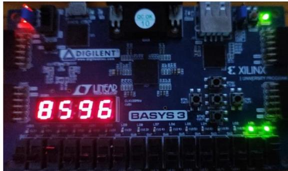
Figura 108. Esclavo - Cpol = 0 Cpha = 1, 16 bits.
