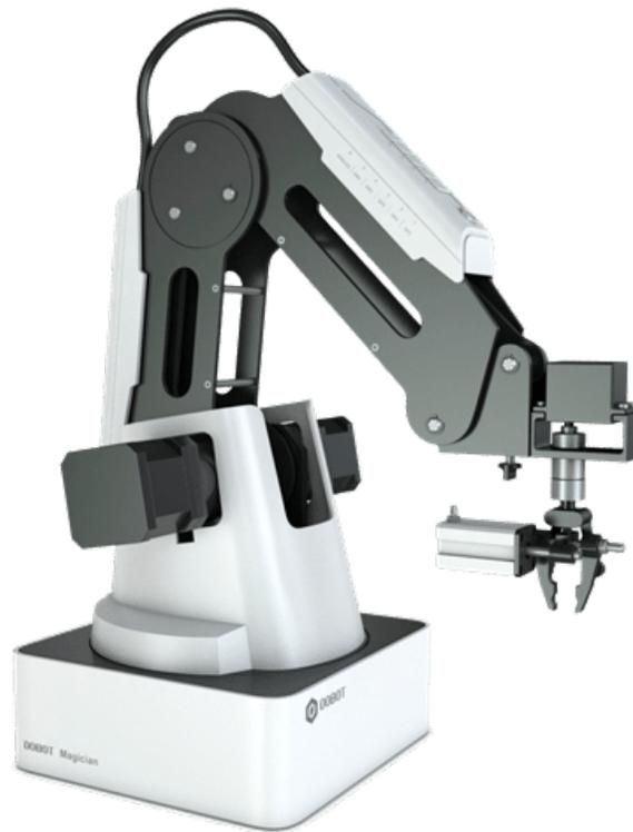
Figura 2.8 Brazo robótico Dobot Magician
