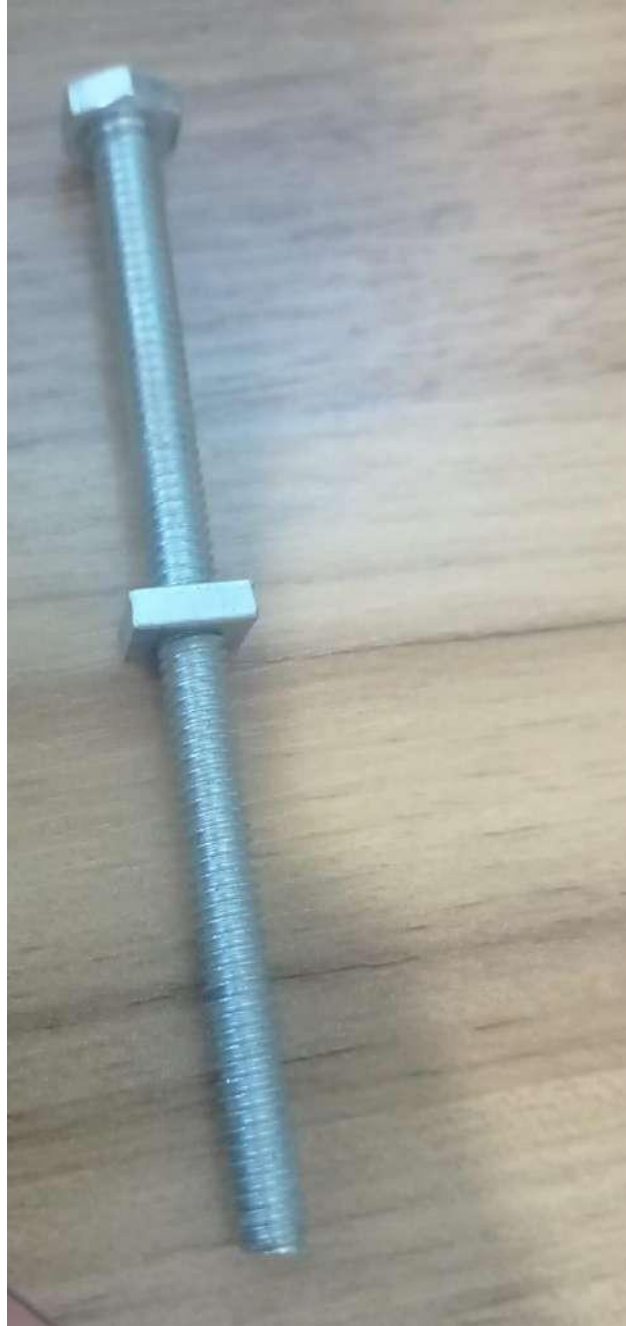
Figure 6.29: Bolts for attaching the gearbox. Source: own
