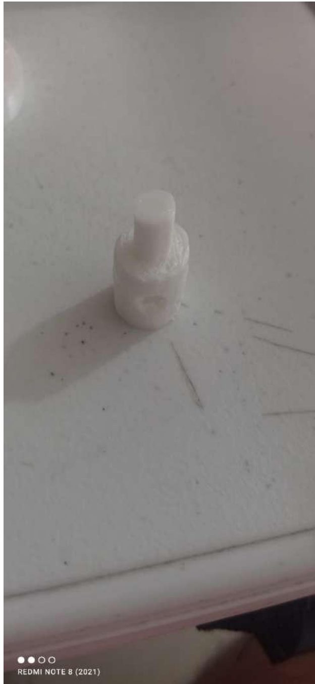
Figure 6.15: 3D printed screw adapter for the motor. Source: own
