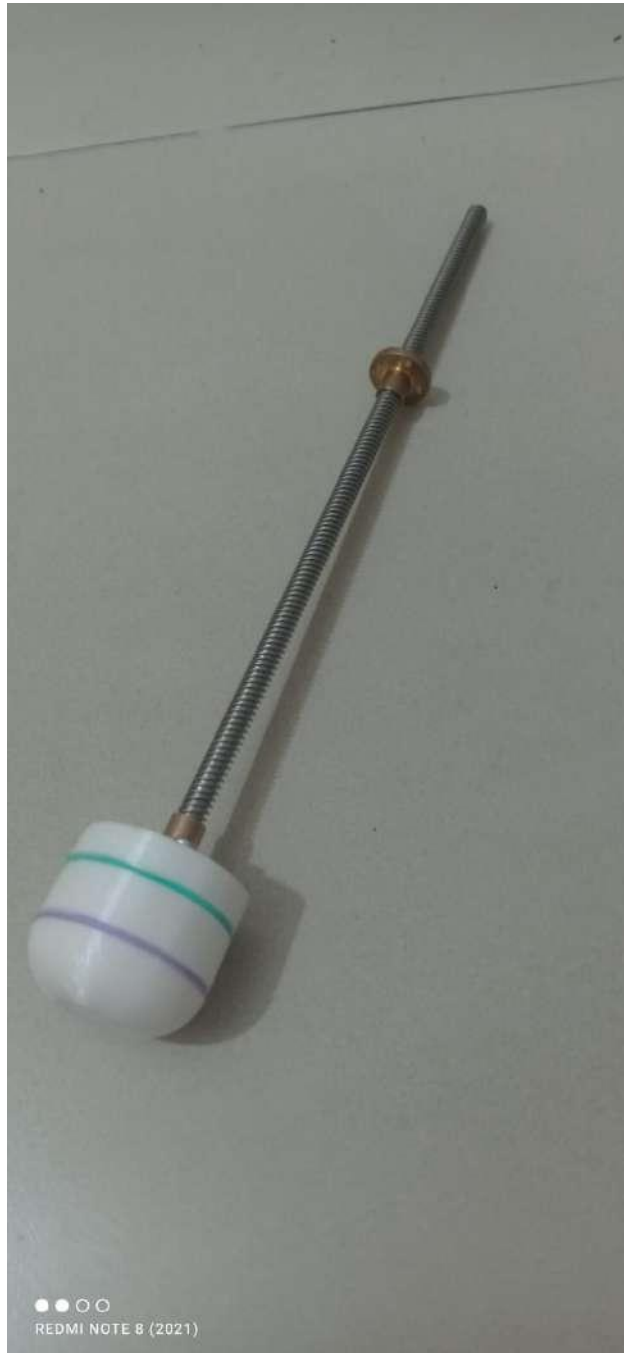
Figure 6.39: Printed plunger connected to the lead screw. Source: own
