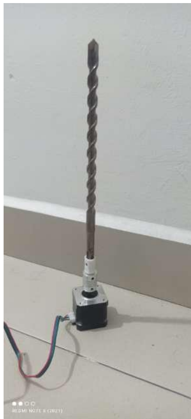
Figure 6.19: Motor and screw assembly. Source: own
