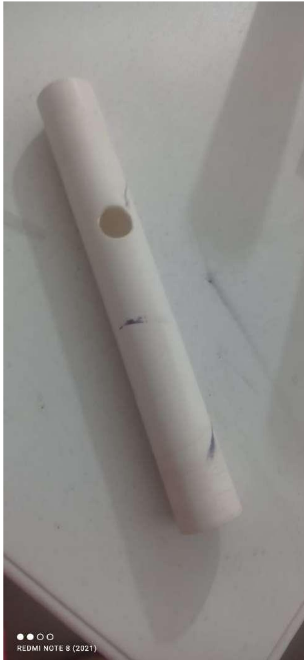
Figure 6.16: PVC with the adapted hole. Source. own
