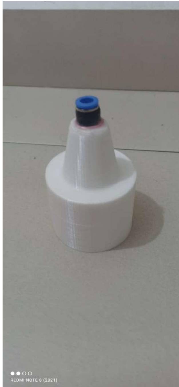
Figure 6.37: Nozzle with two way fitting. Source: own
