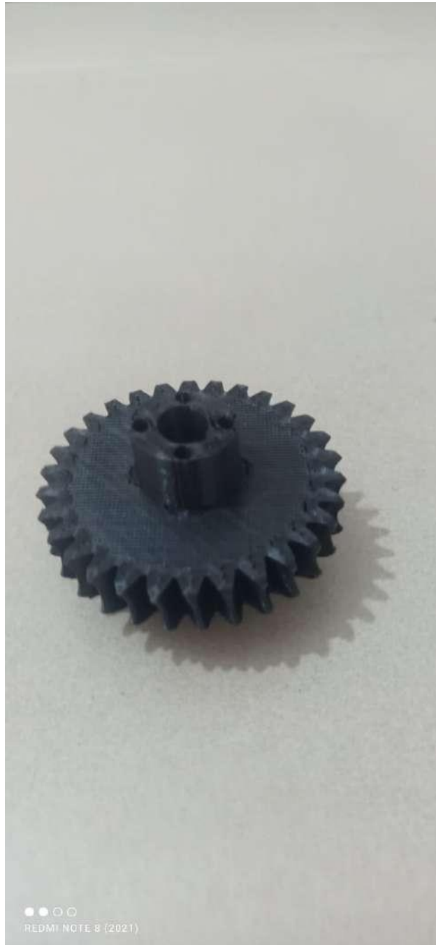
Figure 6.42: Crown gear for the worm-gear assembly. Source: own
