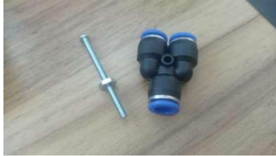
Figure 6.18: Pneumatic fitting for hose and screw-nut pair. Source: own
