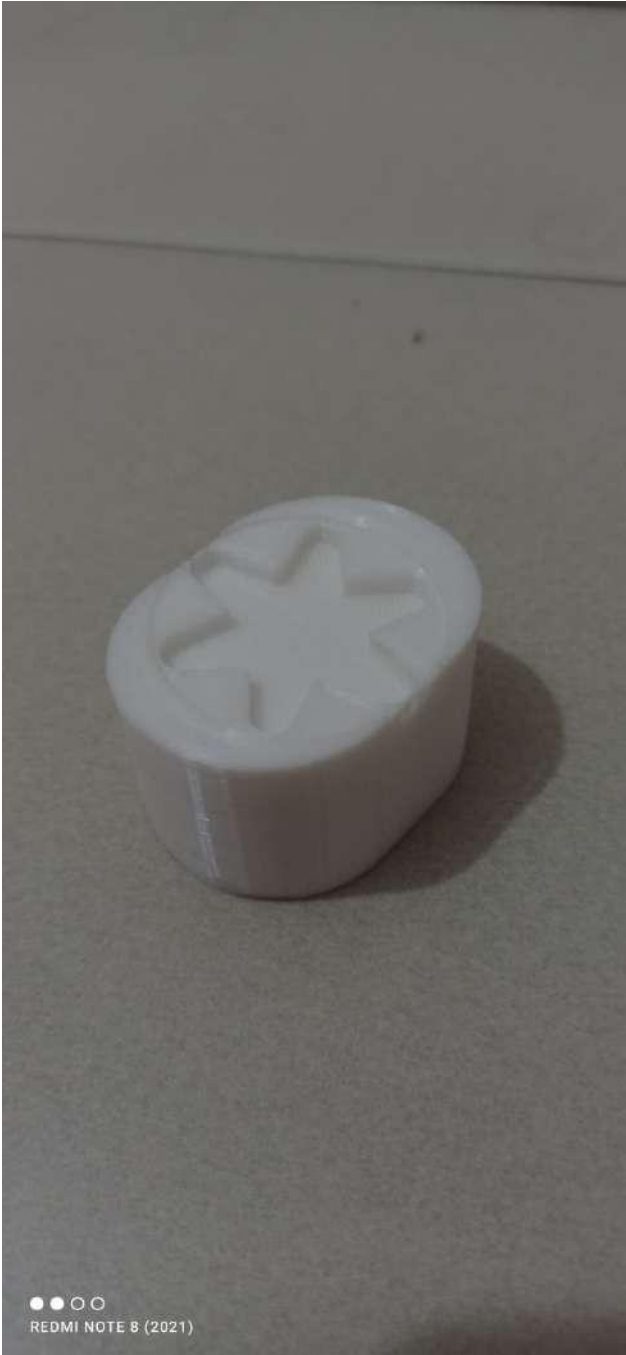
Figure 6.49: Shaft adapter of the servo to the valve. Source: own
