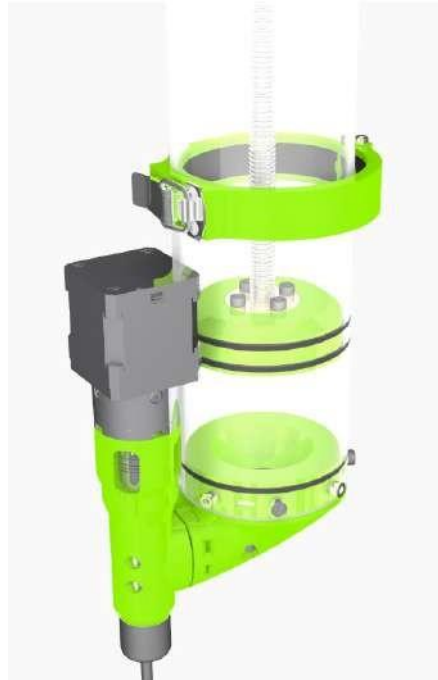
Figure 4.22: CeraStruder configuration. Source: (CeraStruder , n.d.)
