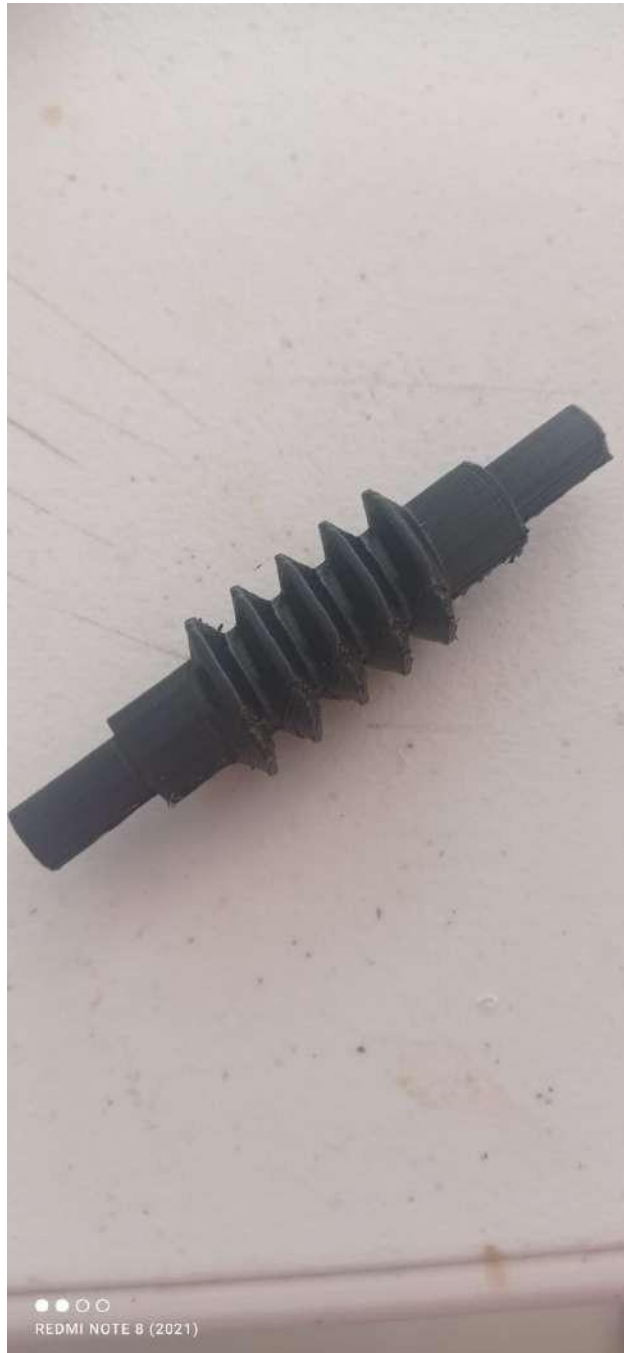
Figure 6.43: Worm for the worm-gear assembly. Source: own
