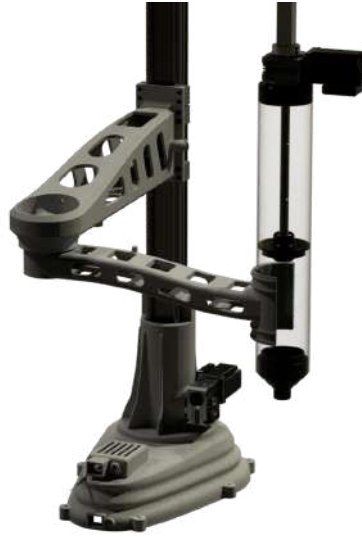
Figure 4.25: 3D Potter extruder. Source: (3D Potterbot Scara V4 ceramic 3D clay printer — real clay 3D ceramic printer , n.d.)
