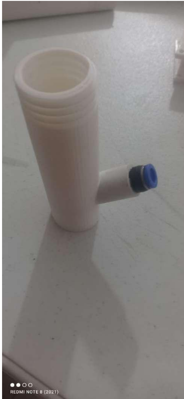
Figure 6.13: 3D printed top part. Source. own
