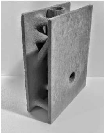
Figure 4.16: Wall-element with integrated tube, additive manufactured by selective cement activation. Source: (Kloft et al., 2021)
