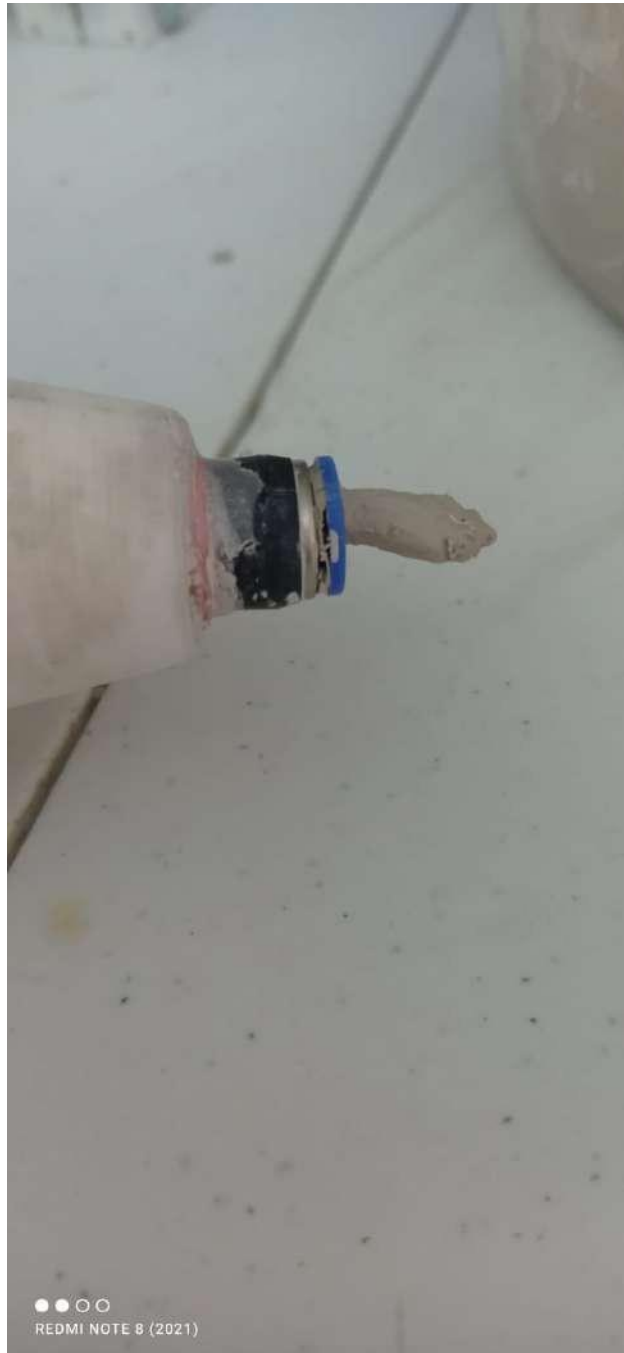
Figure 7.6: Shape of the clay extrusion in the feeder. Source:own
