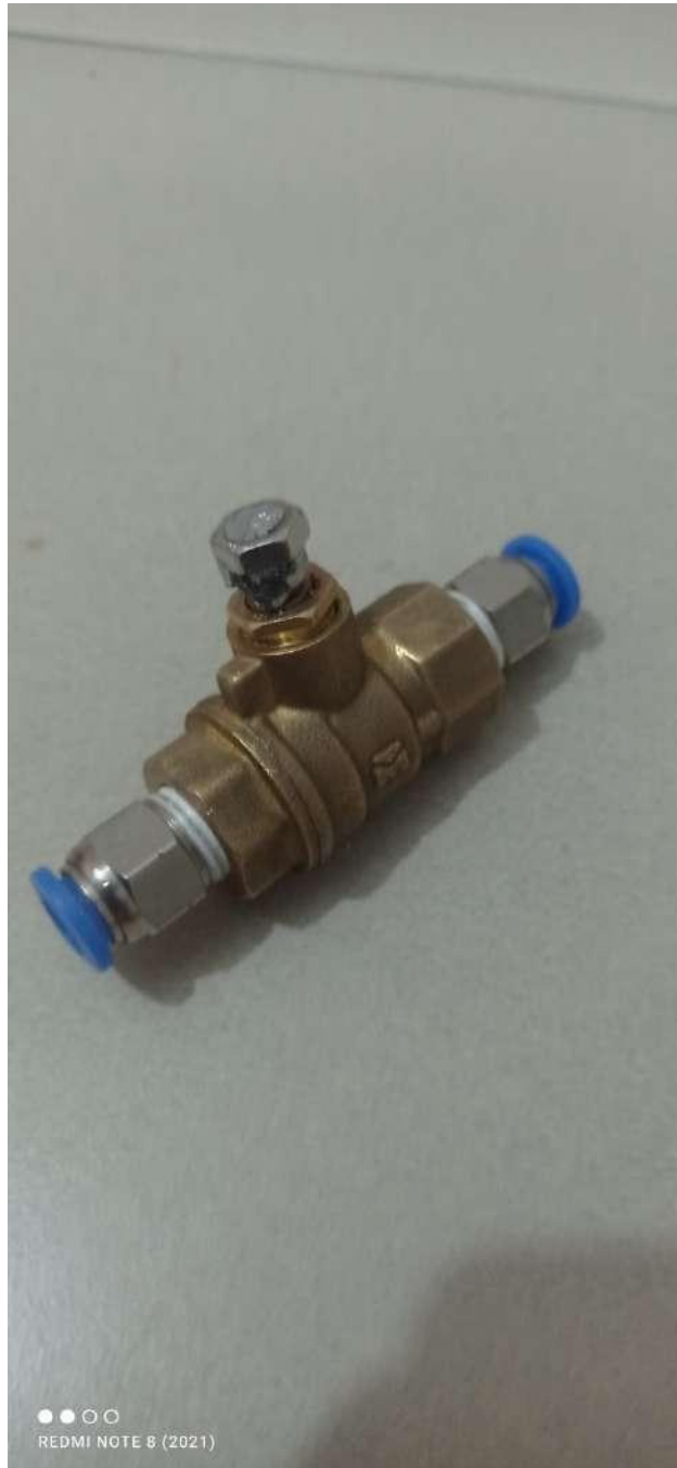
Figure 6.50: Modified valve to fit the shaft adapter. Source: own
