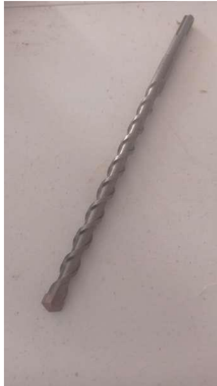
Figure 6.6: Drill bit used as a extruder. Source: own
