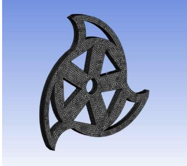
Figure 5.1: Mesh of the blade in ANSYS. Source: own
