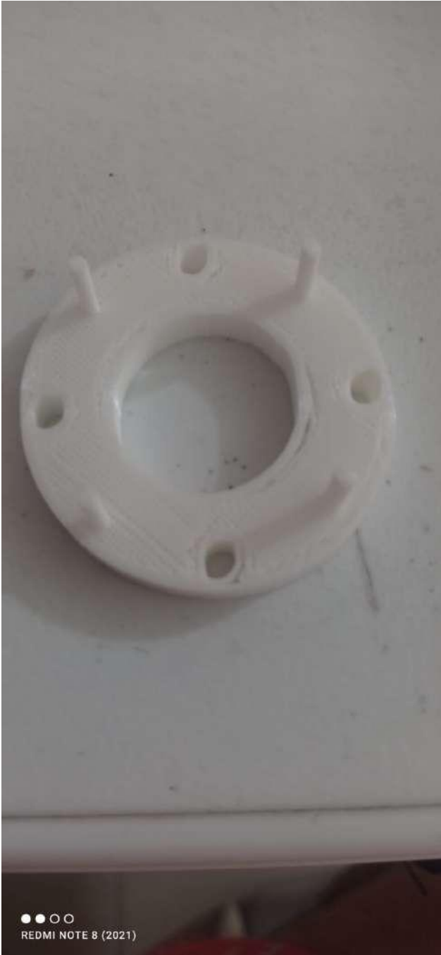
Figure 6.14: 3D printed motor support. Source: own
