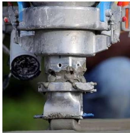
Figure 4.33: COBOD extruder. Source: (The BOD2 , 2023)
