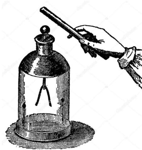
Figura 1.1 Electroscopio [3]
