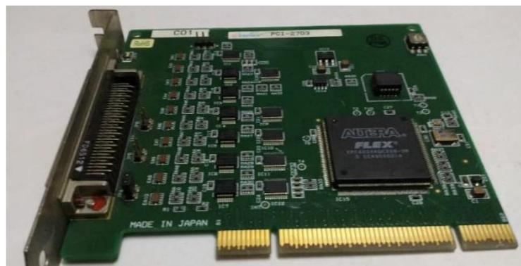
Figura 5.2 Tarjeta PCI 2703A
