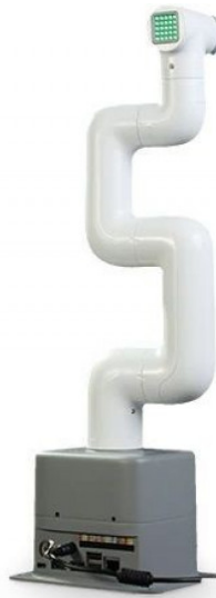
Figura 4.1: Brazo robótico MyCobot 280 Jetson Nano. Obtenida de: https://top3dshop.com/product/elephant-robotics-mycobot-280-jetson-nano
