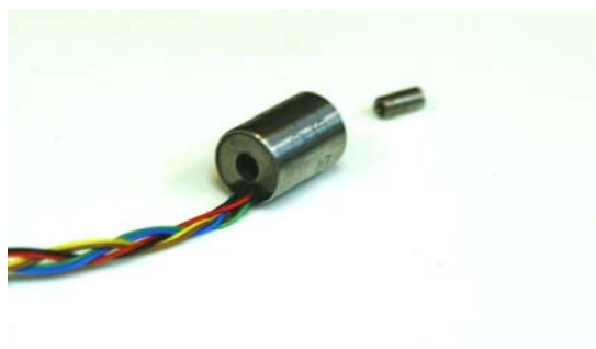
Figura 3.4 LVDT (Linear Variable Differential Transformer)
