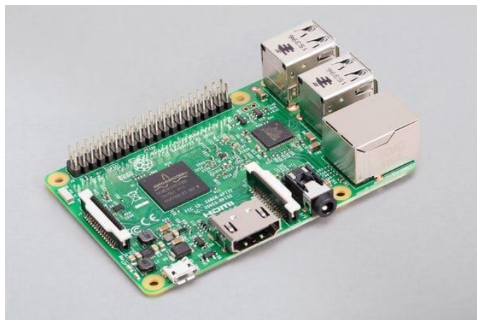
Figura 6.1.1: Raspberry Pi 3 Versión B. Tomado de "Raspberry Pi 3 Model B" por Local Raspberry Pi, https://www.raspberrypi.com/products/raspberry-pi-3-model-b/
