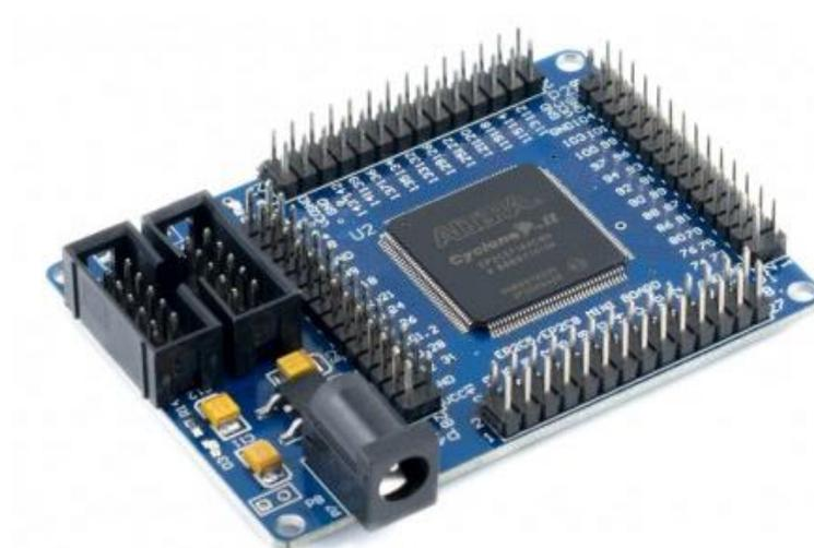
*Figura 1.2 FPGA Cyclone II de ALTERA*
