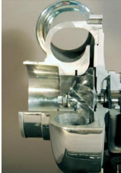
*Figura 4.55: Corte transversal de un compresor. [ TURBO Real World High-Performance Turbocharger Systems. (p.18), por Miller, J. (2008) North Branch, Car Tech].*
