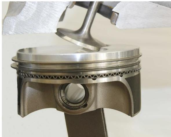
*Figura 4.4: Valve Reliefs, por Smith,J, 2018, <https://www.hotrod.com/articles/measuring-setting-valve-piston-clearance-advanced-guide/>*
