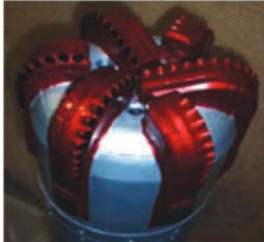
*Figura 28. Barrena convertible (Aguilera, L. et al., 2013)*
