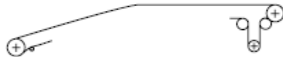
Figure 2.4 Ascending and horizontal path, when belt tensions will permit one belt and space will permit vertical curve.
