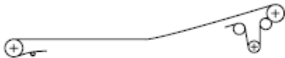
Figure 2.3 Horizontal and ascending path, when space will permit vertical curve and belt strength will permit one belt.
