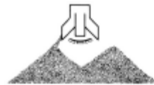
Figure 2.14 Discharge from tripper to one side only, to both sides, or forward again on conveyor belt.
