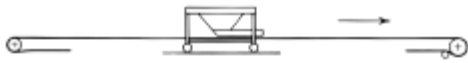
Figure 2.10 Traveling loading chute to receive materials at a number of points along conveyor.
