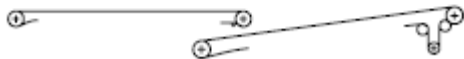
Figure 2.5 Possible horizontal and ascending path, when space will not permit a vertical curve or when the conveyor belt strength requires two belts.
