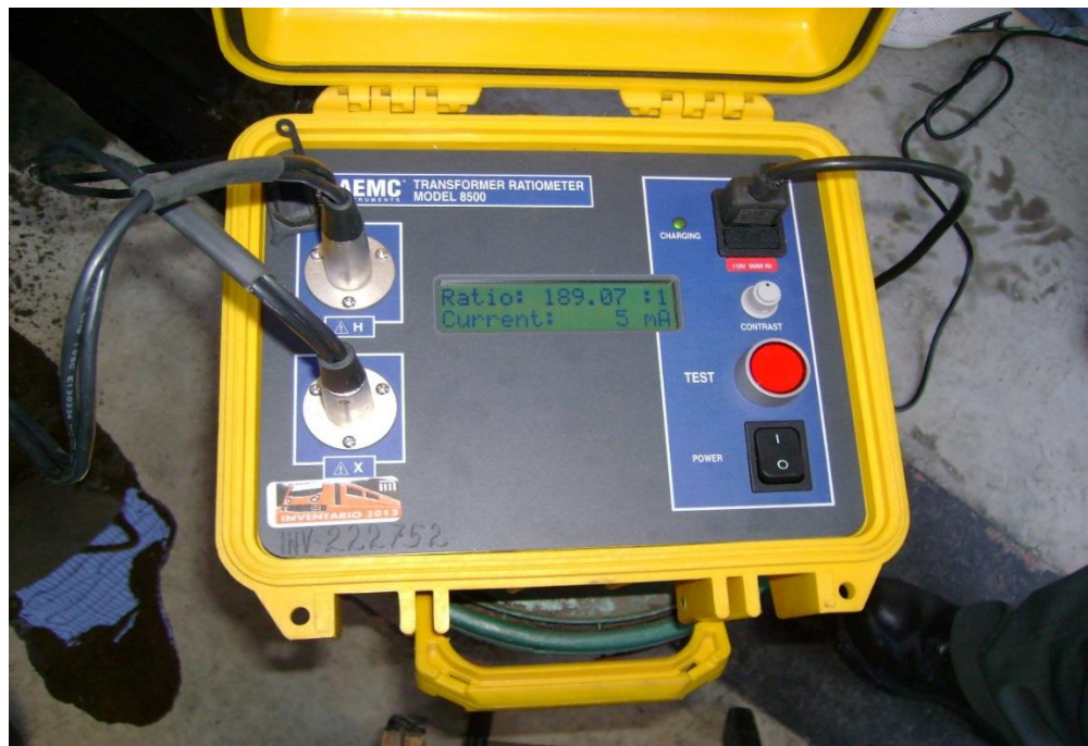
Figura 4-2 Digital Transformer Ratiometer DTR Mod. 8500 de AEMC INSTRUMENTS.
