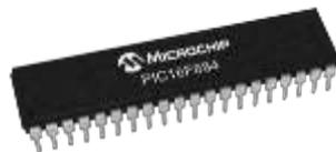
**Fig. 48.** Microcontrolador PIC 16F884 de Microchip. [29]
