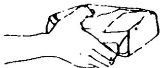
Hold the option (still wrapped in its anti-static bag) in one hand and touch a metal part of the system unit with the other hand. This will place your body, the option, and the system unit at the same ground potential, thus preventing an accidental static discharge.
