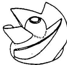
(e) MIXED VANE 10,000 gpm to 30,000 gpm
