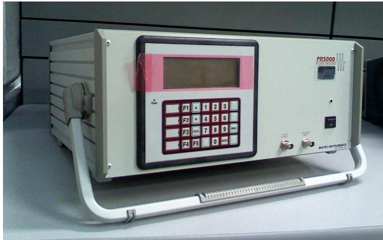
Fig 5.2. Pulsador/Receptor Matec PR5000.
