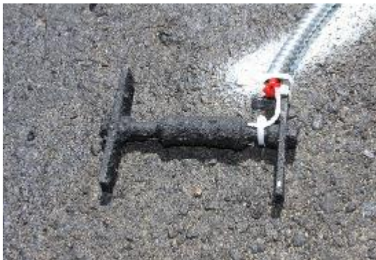
SENSORES ASG (Asphalt Strain Gages)
