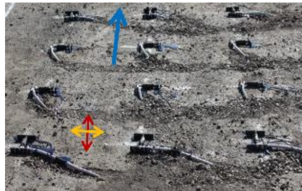
SENSORES ASG (Asphalt Strain Gages)
