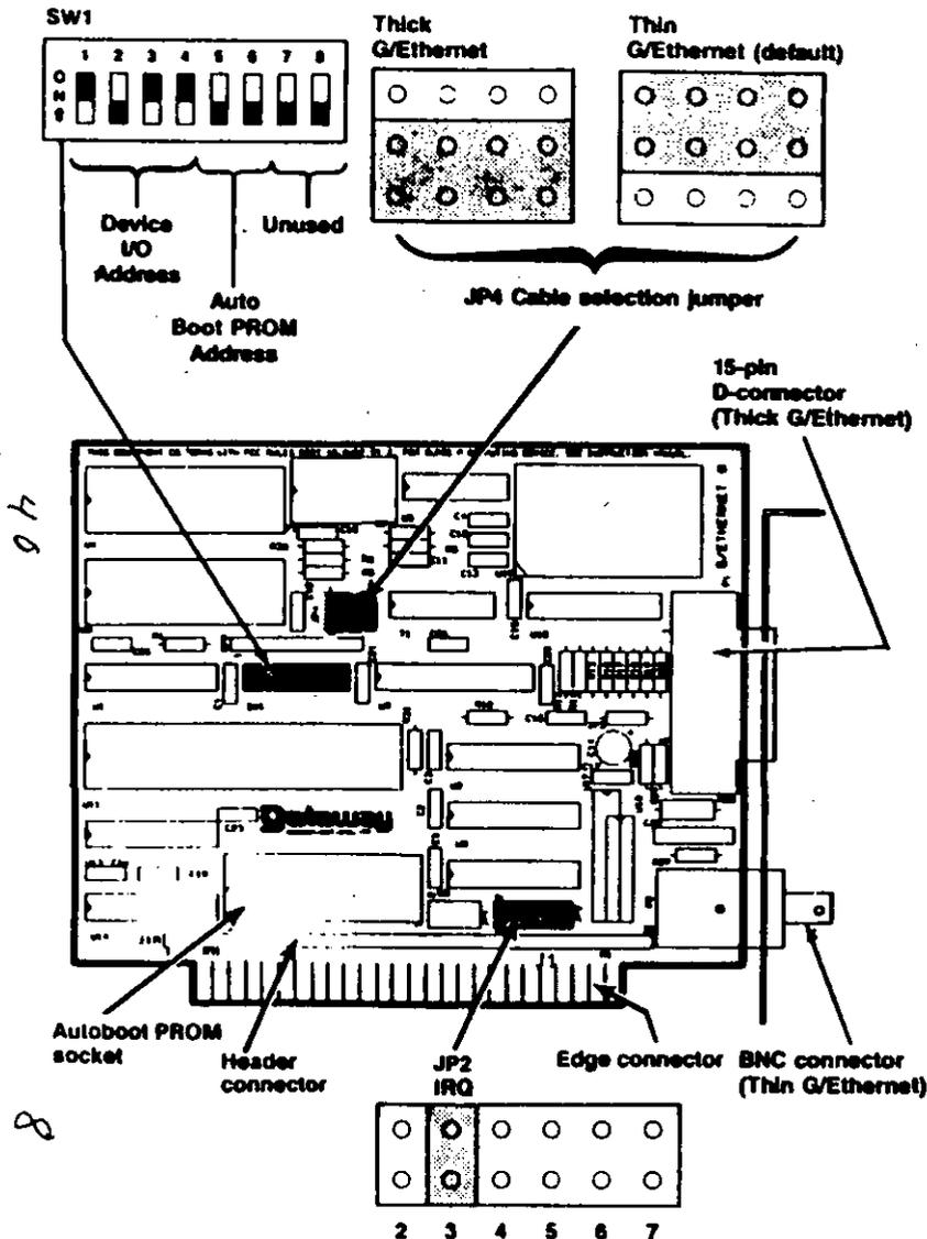
Figure 2-1. G/Ethernet 16-bit Component Locations.
