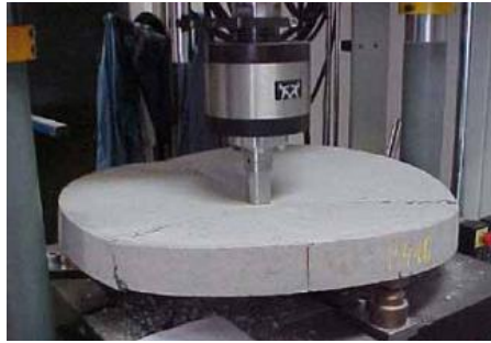
Figura 1.7 Ensayo de panel circular (ASTM C1550)
