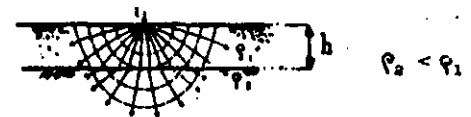
Figure 7. Current and potential patterns for uniform soil with protective surface layer of high resistivity.
