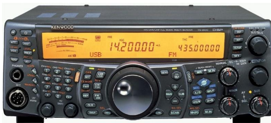
Figura 5-16 Transceptor modelo TS-2000X 23
