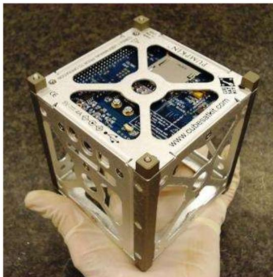
Figura 1-3 Estructura CubeSAT [6]
