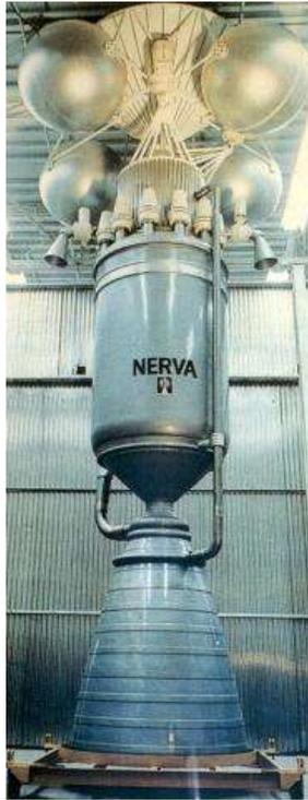
**Figura 3-16 Propulsor nuclear NERVA-1 [39]**
