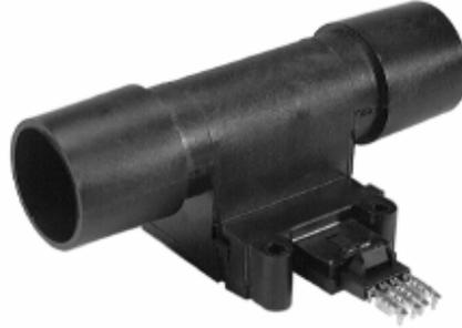
AWM700 Series microbridge mass airflow sensors provide in-line flow measurement with a specially designed bypass flow housing. The sensors measure flow as high as 200 standard liters per minute (SLPM) while inducing a pressure drop of 1 inch H<sub>2</sub>O, typically. The AWM700 has a high flow range capability in a small package.
