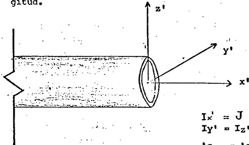
$$\begin{aligned} I_{x'} &= J \\ I_{y'} &= I_{z'} = I \\ A_{c_{y'}} &= A_{c_{z'}} = A_c \end{aligned}$$
