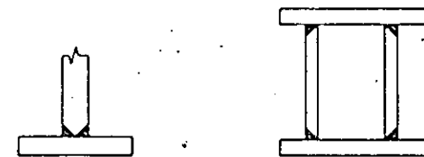
Fig. 5.5.3. Uses of groove welds in tee joints.
