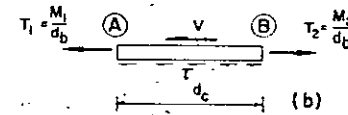
FIG. 8.17b.—FREE BODY DIAGRAM OF FORCES ACTING ON TOP STIFFENER AND COLUMN WEB
